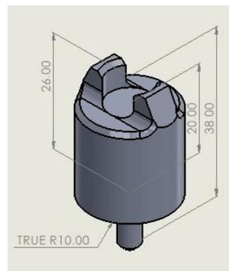
**Figure 7.** Marble support used in the track.
