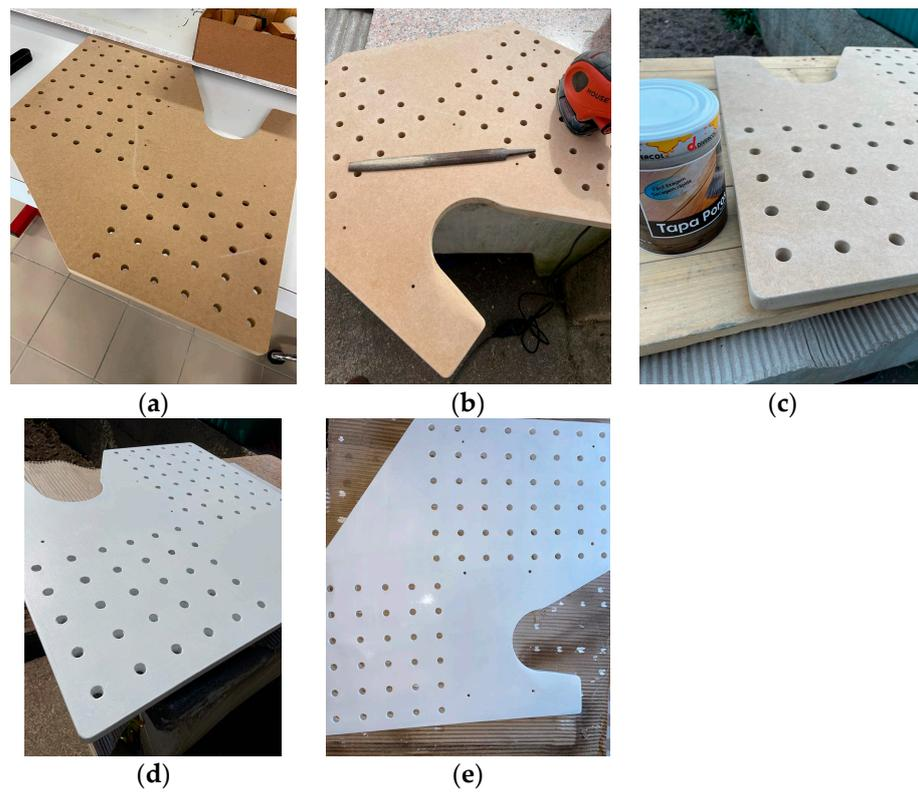
**Figure 5.** Treatment process: (a) raw wooden board; (b) sanding the wooden board; (c) application of pore filler on the board; (d) application of paint on the board; and (e) application of matte varnish on the board.
