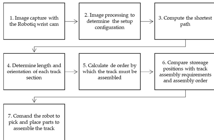
**Figure 17.** Program flowchart that enables track analysis and assembly.
