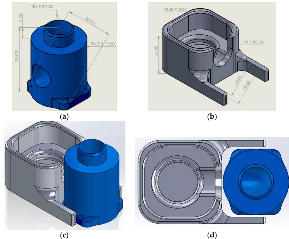
**Figure 12.** (a) Transport component. (b) Final component. (c) Fitting of the final component and the transport piece. (d) Top view of the fitting of the final component and the transport piece.
