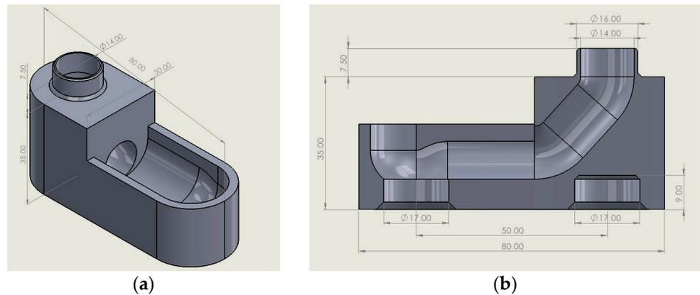
**Figure 11.** (a) Track section 1. (b) Fittings of track section 1.
