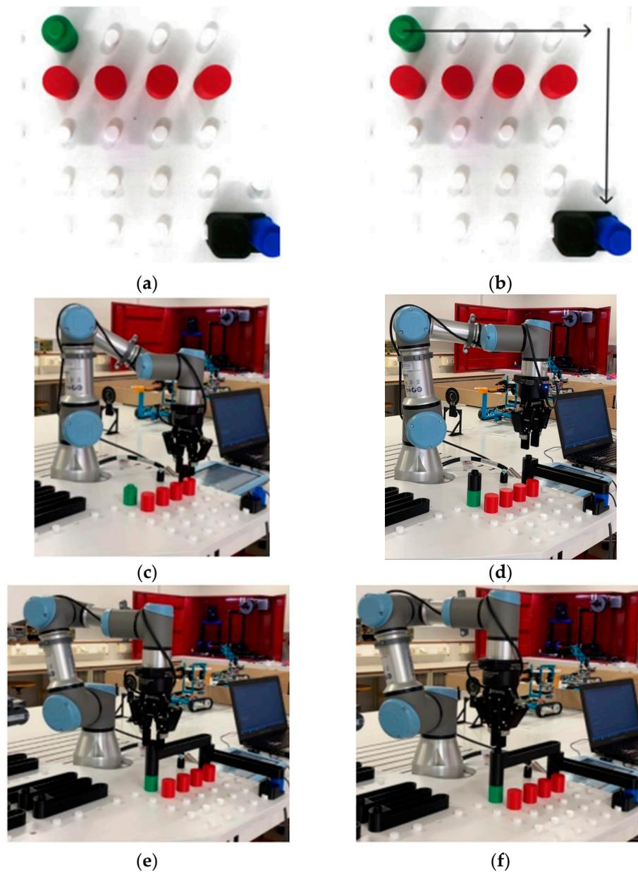
**Figure 19.** Movement sequence of Protocol 2—track with two straight sections and one curve. (a) Setup example. (b) Shortest path. (c) Assembly level 1. (d) Assembly level 2. (e) Assembly level 3. (f) Placing the marble to travel.
