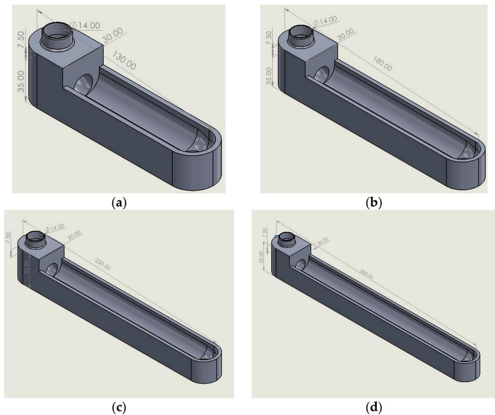
**Figure 13.** Version 2 of the track sections: (a) track section 2, (b) track section 3, (c) track section 4, and (d) rack section 5.
