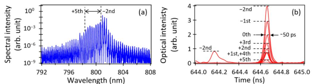
**Figure 5.** (a) Power spectrum of the MMLD output corresponding to the temporal waveform in Figure 4b. (b) Temporal waveforms of the MMLD output for the respective (the negative second to the fifth) modes.
