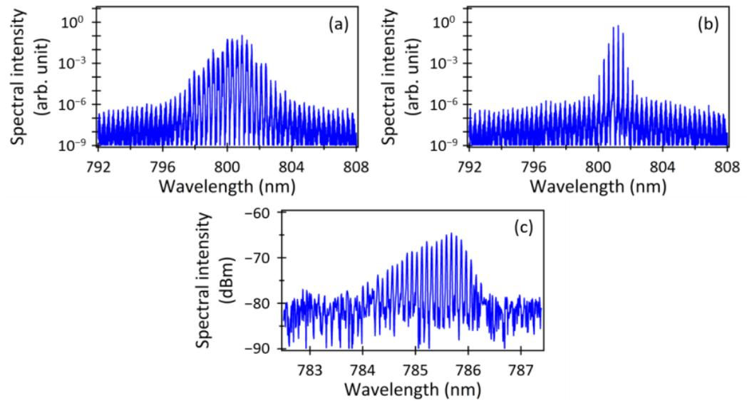
**Figure 6.** (a,b) Power spectra calculated using the temporal waveforms shown in Figure 4c,d, respectively. (c) Experimentally observed power spectrum of the output from the MMLD with delayed optical feedback [30].
