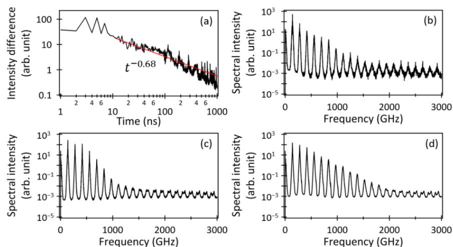
**Figure 8.** (a) Temporal variation in the intensity difference between the adjacent averaged THz-TDS output spectra. Examples of the THz-TDS output spectra averaged over (b) 10 ns, (c) 100 ns, and (d) 500 ns, respectively.
