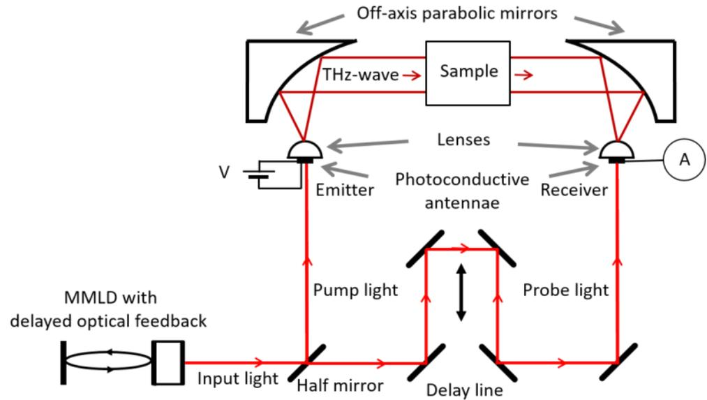
**Figure 1.** Configuration of the THz-TDS system using an MMLD with delayed optical feedback.
