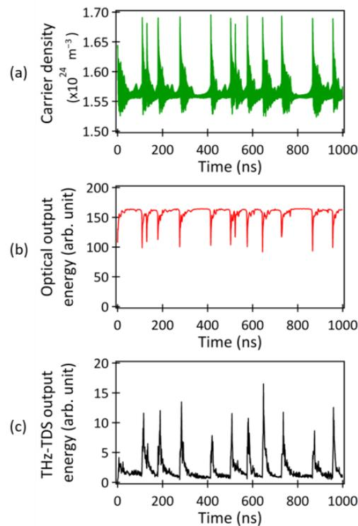
**Figure 3.** (a) Temporal waveform of the carrier density when  $f_c$  was set to 0.4. The temporal variations in the (b) MMLD output energy and (c) THz-TDS output energy integrated every 1 ns.
