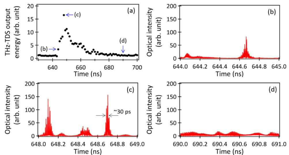
**Figure 4.** (a) A magnified view of a section from Figure 3c. The temporal waveforms of the MMLD outputs are shown during the time periods (b) 644–645 ns, (c) 648–649 ns, and (d) 690–691 ns, respectively.
