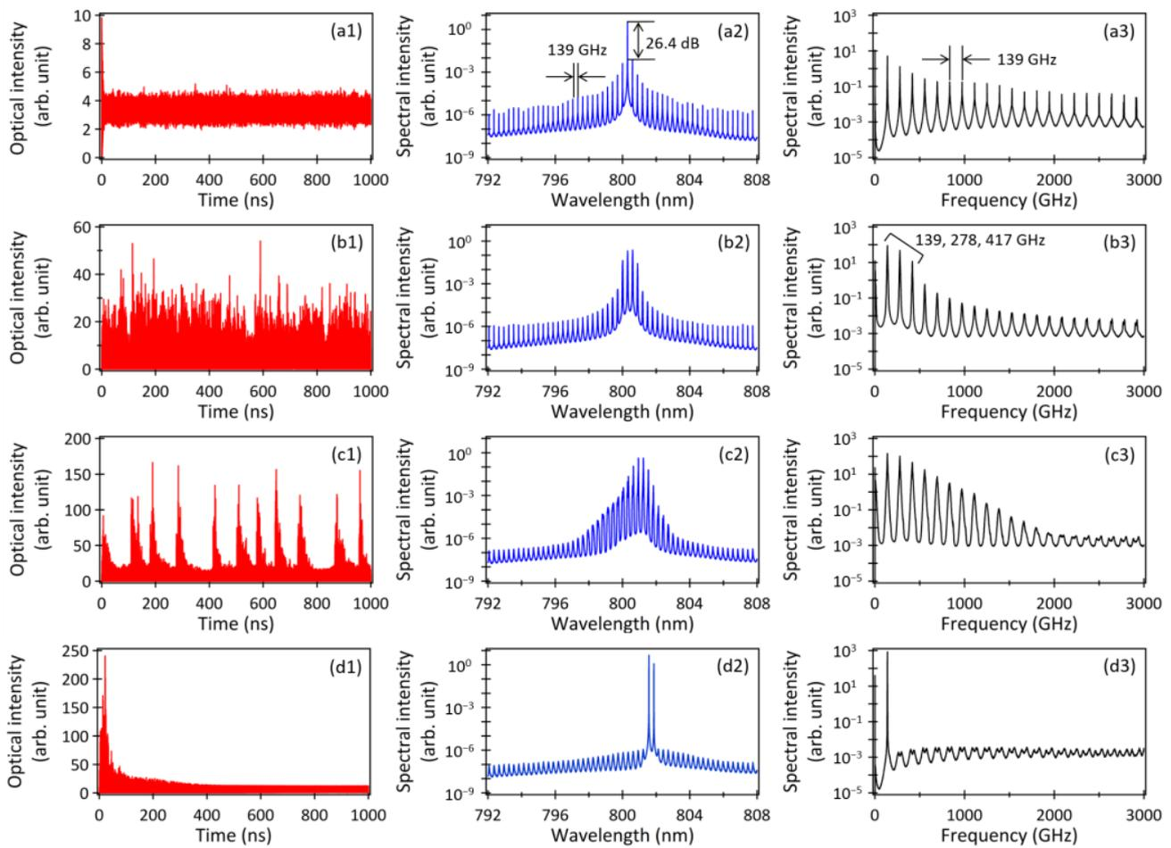
**Figure 2.** Temporal waveforms of the MMLD outputs (a1–d1), along with the corresponding power spectra (a2–d2) and THz-TDS outputs (a3–d3) for the different values of  $f_c$  (0 (a1–a3), 0.1 (b1–b3), 0.4 (c1–c3), and 0.6 (d1–d3)). The parameters  $r$  and  $\tau_{fb}$  were set to 1.5 and 1 ns, respectively.
