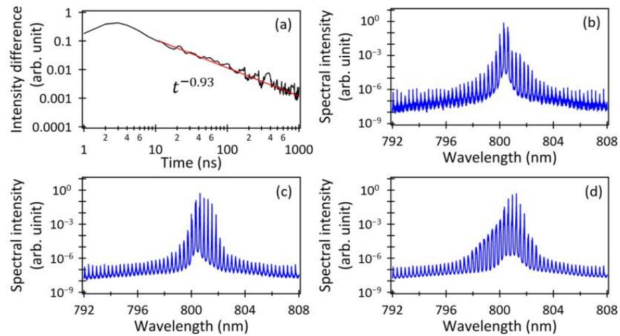
**Figure 7.** (a) Temporal variation in the intensity difference between the adjacent averaged MMLD output spectra. Examples of the MMLD output spectra averaged over (b) 10 ns, (c) 100 ns, and (d) 500 ns, respectively.
