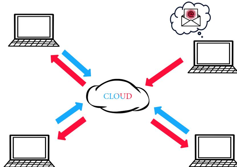
**Figure 1.** This figure illustrates the VirLock cloud storage spread and infection. In this example, the user of the top right computer opened a malicious email attachment that infected the PC with the VirLock malware. The files in the network share of the cloud storage will also become infected. The malware may eventually spread to other machines in the network. The blue arrows represent interaction with the cloud, while the red ones show the route of the infection.
