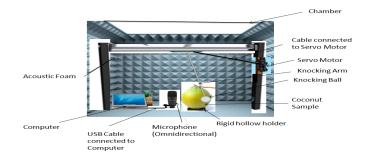
**Figure 1.** The system with coconut fruit and signal acquisition [1].
