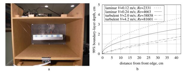
**Figure A2.** (a)  $\varepsilon = 3$  mm plate in wind-tunnel; (b) wind-tunnel boundary layers.
