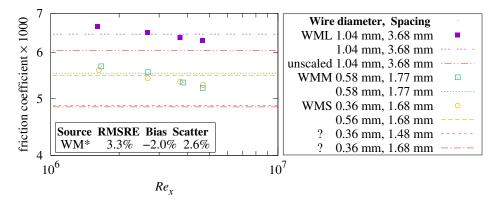
**Figure 21.** Local  $f_{\rho}$  versus  $Re_x$  of woven wire mesh [13].
