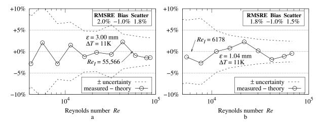
**Figure A6.** (a) Measured versus theory  $\varepsilon = 3$  mm; (b) Measured versus theory  $\varepsilon = 1$  mm.
