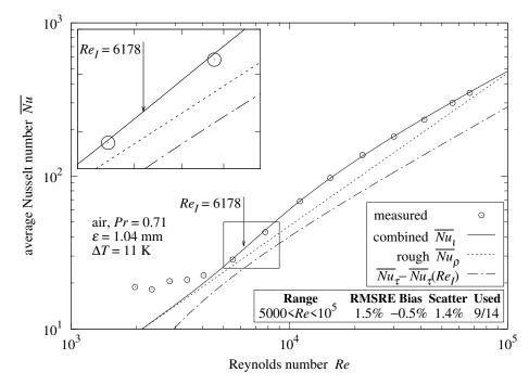
**Figure 24.** Convection from bi-level plate;  $L/\varepsilon = 295$ .
