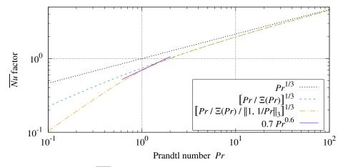
**Figure 13.** Smooth plate  $\overline{Nu_{\tau}}$  dependence on *Pr*.
