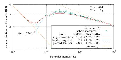
Figure 26. Average friction versus *Re* of smooth plate [20,21].
