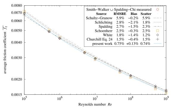
**Figure 7.** Average  $\overline{f_{\tau}}$  versus *Re* of smooth plate, [11].
