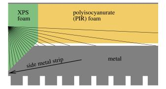
Figure A5. XPS wedge conduction.
