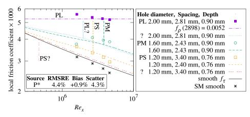
**Figure 22.** Local  $f_{\rho}$  versus  $Re_x$  of perforated sheet [13].
