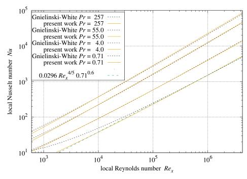
Figure 16. Smooth plate local turbulent convection.
