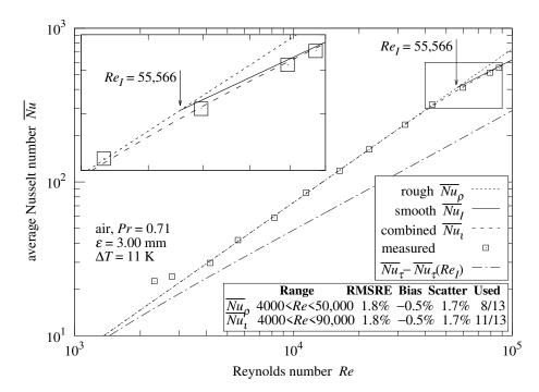
**Figure 23.** Convection from bi-level plate;  $L/\varepsilon = 102$ .
