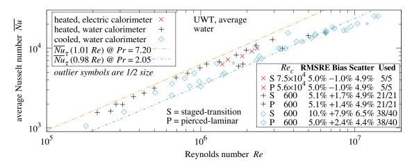
Figure 37. UWT average convection in water [18].
