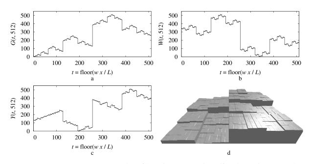
**Figure 3.** (a) Gray -code profile roughness; (b) wiggliest self-similar roughness; (c) random reversal profile roughness; (d) random reversal ramp surface.
