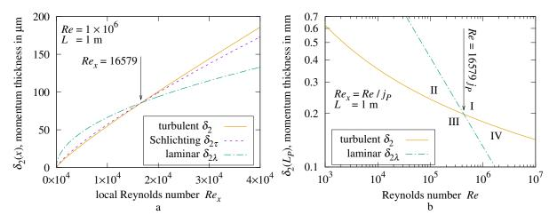
**Figure 17.** (a) smooth plate  $\delta_2(x)$  versus  $Re_x$ ; (b) Smooth plate  $\delta_2(L_P)$  versus Re.
