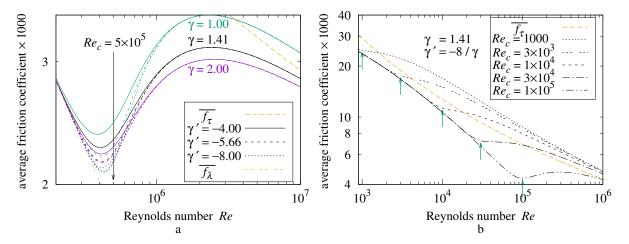
**Figure 25.** (a) Pierced-laminar friction by  $\gamma$ ,  $\gamma$ '; (b) Pierced-laminar friction by  $Re_c$ .
