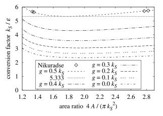
**Figure 2.**  $k_S / \varepsilon$  versus cell area of sand-roughness [4].
