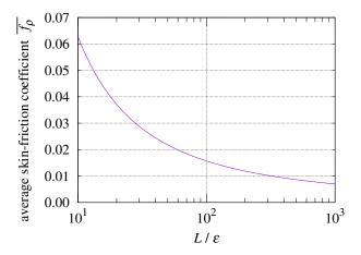
**Figure 5.** Average  $\overline{f_{\rho}}$  versus  $L/\varepsilon$  of rough plate.
