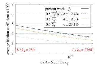
Figure 10. Average friction coefficient of sand-roughness.
