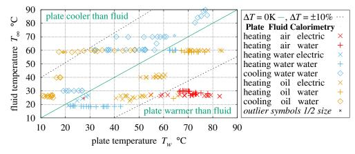
Figure 34. UWT plate-fluid temperature pairs [18].
