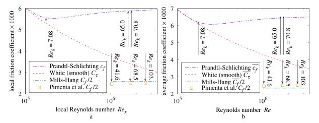
**Figure 1.** (a) Local  $c_f$  versus  $Re_x$  [8], (b) Average  $\overline{c_f}$  versus Re.
