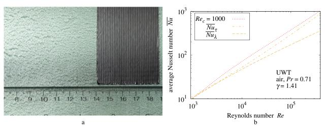
Figure 27. (a) XPS foam board and duck tape; (b) duck tape convective heat transfer.
