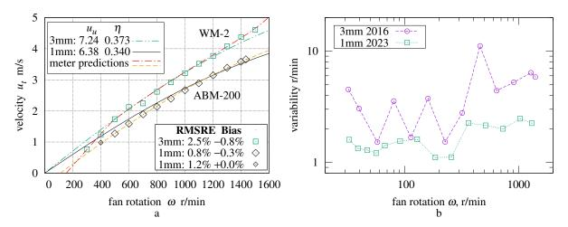
Figure A3. (a) Airspeed versus fan speed; (b) Fan PLL variability.
