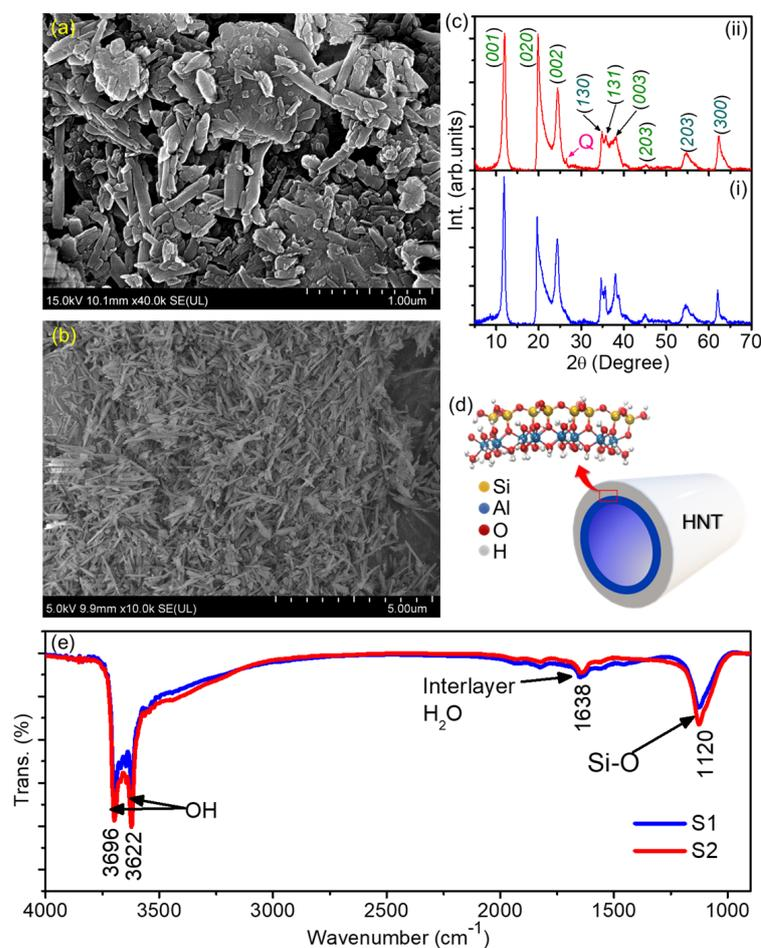
**Figure 2.** FESEM images of (a) S1 and (b) S2 sample. (c) Schematic of HNT depicting its structure and possible chemical composition. (d) XRD profile of (i) S1 and (ii) S2. The label “Q” in panel (ii) indicates minor contribution from quartz impurities. (e) FTIR spectra of S1 and S2 samples.
