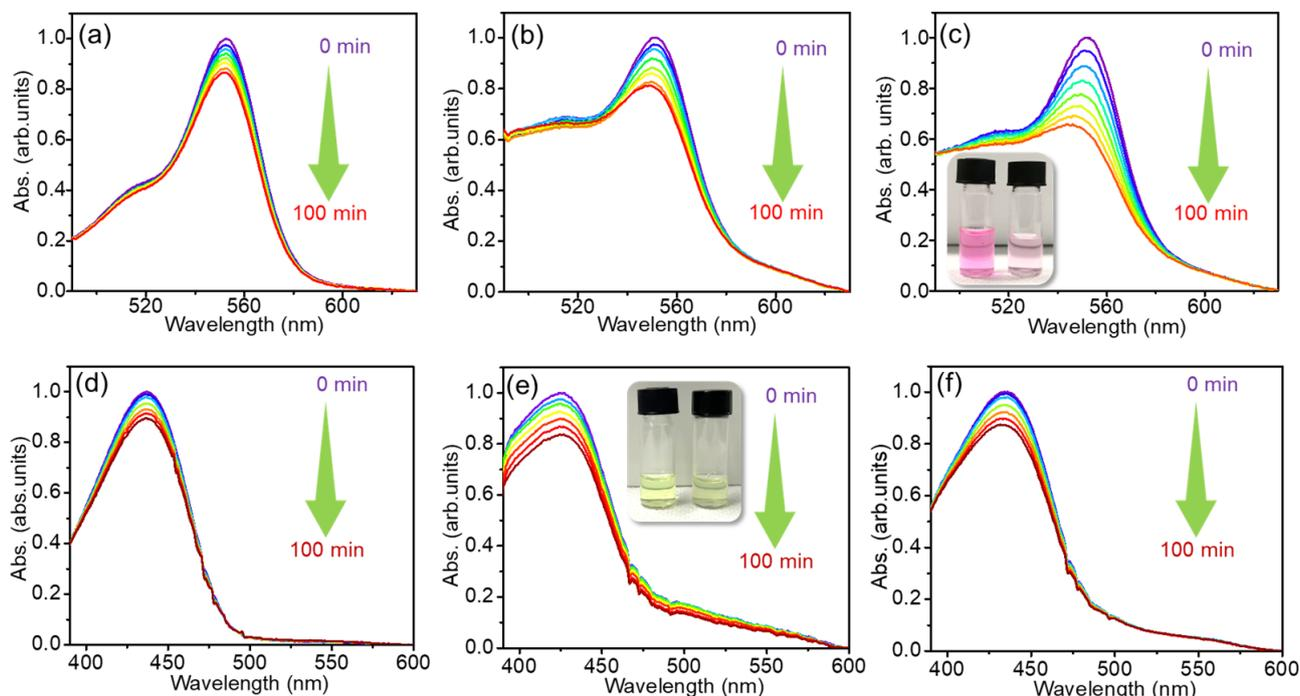
**Figure 3.** Absorption spectra of (a) bare cationic RhB, and RhB in the presence of (b) S1 and (c) S2 under UV-Visible light irradiation as a function of exposure time; inset of panel (c): digital image of RhB dye before and after degradations. Absorption spectra of bare (d) anionic C343 dye, and C343 in the presence of (e) S1; inset of figure (e): digital image of C343 dye before and after degradations, and (f) S2 under the UV-Visible light irradiation.
