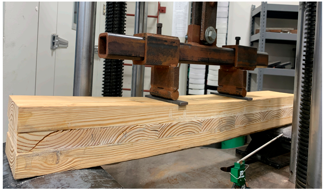
Figure 4. Rolling shear failure in non-densified CLT samples.
