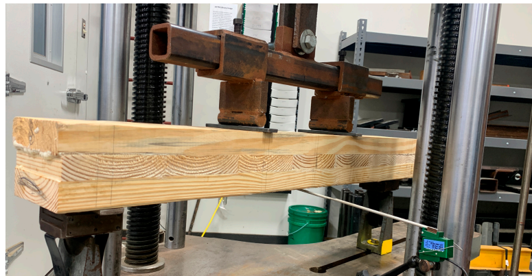
Figure 1. Third-point bending set-up as per ASTM D198.
