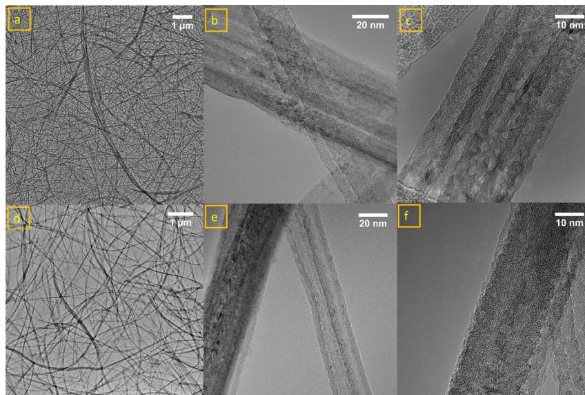
**Figure 2.** TEM images of TiNTs (**a–c**) and 1.0 wt% Fe/TiNTs (**d–f**).
