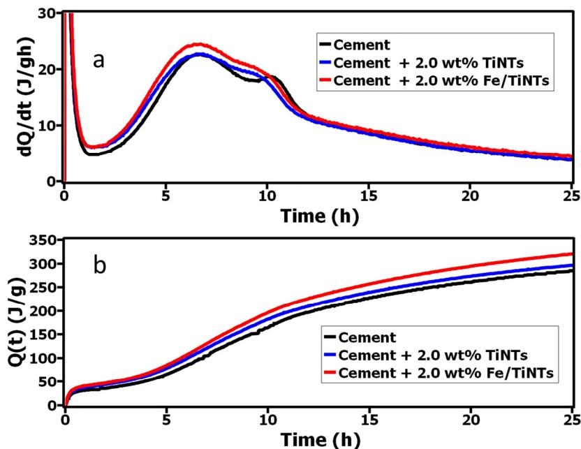
**Figure 9.** Heat evolution (a) and cumulative heat evolution (b) of OPC in the presence and absence of TiNTs and Fe/TiNTs during the 24 h hydration.
