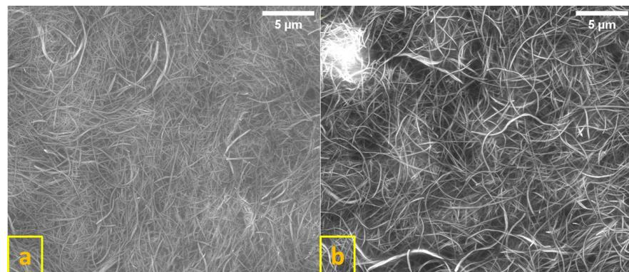
**Figure 1.** SEM images of TiNTs (a) and 1.0 wt% Fe/TiNTs (b).
