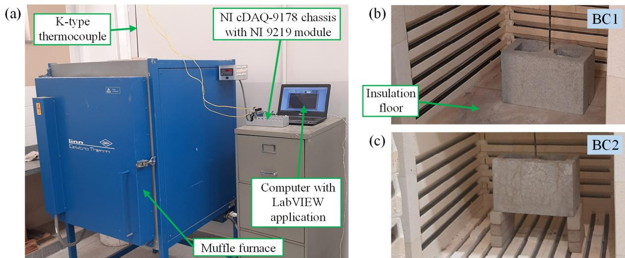
**Figure 2.** Experimental setup used to heat the masonry components (a), according to the BC1 (b) and BC2 (c) configurations.
