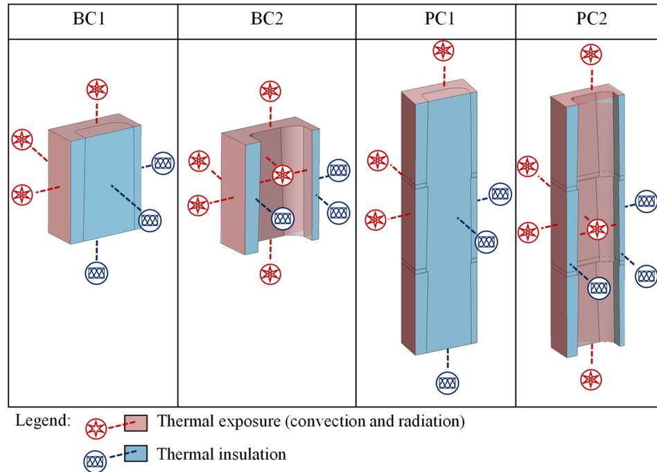
Figure 6. Schematic of the boundary conditions of the finite element models.
