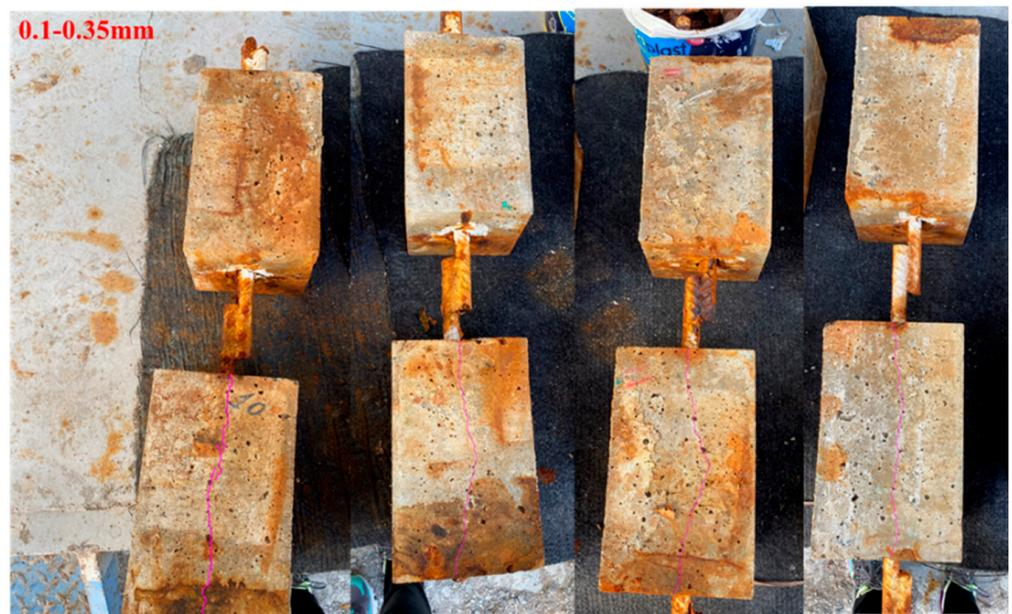
**Figure 3.** Corroded substrates: crack pattern and opening range.
