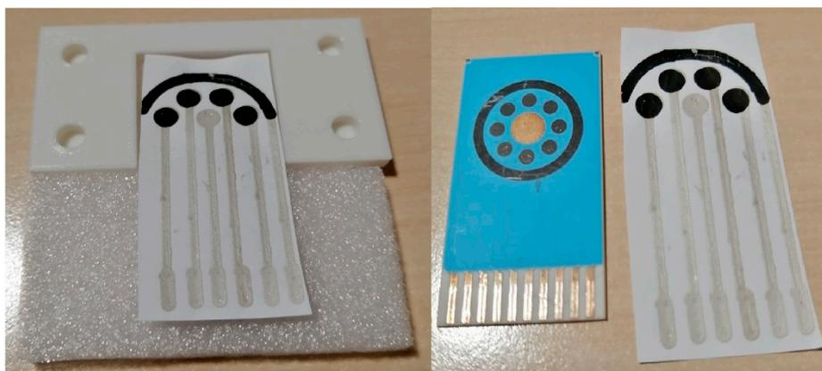
**Figure 3.** Customized functionalization of multi-SPE using 2D printing.
