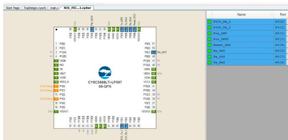
**Figure 5.** Details regarding the PSOC5 configuration.
