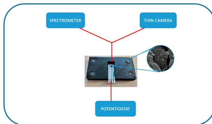
**Figure 1.** Modules of the detection platform.
