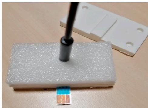
**Figure 9.** Combined electrochemical and optical setup initial prototype.
