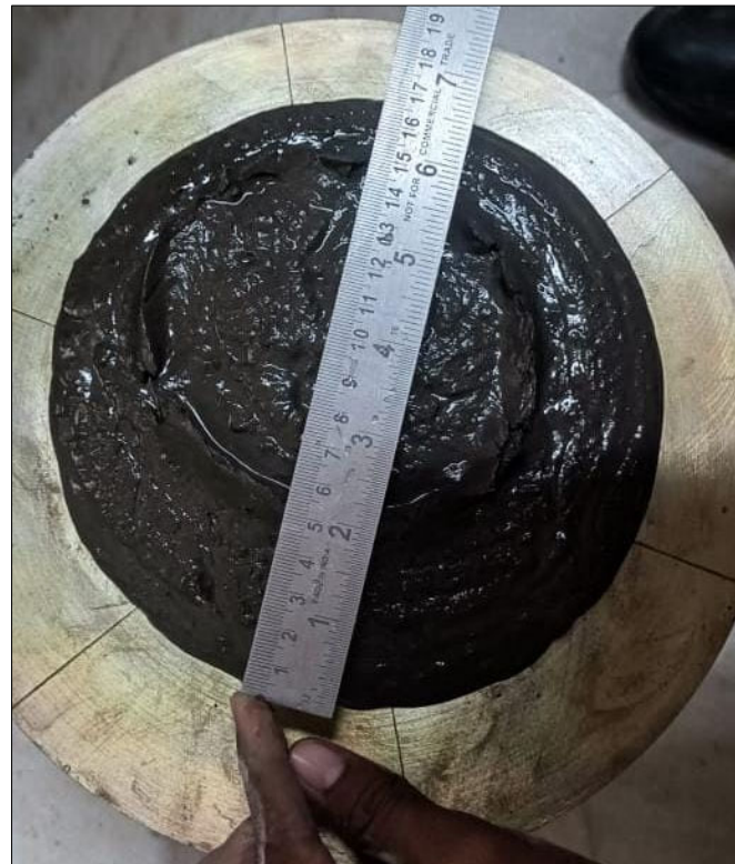
Figure 8. Illustration of the flow table test conducted on mortar.
