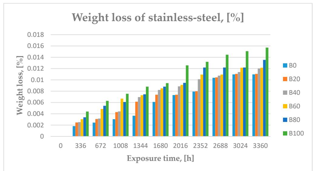
Figure 5. Weight loss of stainless steel plates measured every 336 h for 3360 h, [%].
