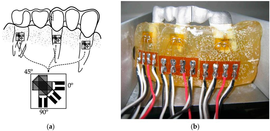
**Figure 9.** Layout of the strain gauges attached to the hemi-jaw: (a) schematic drawing of the layout and the rosette-type strain gauge and (b) image depicting the layout.
