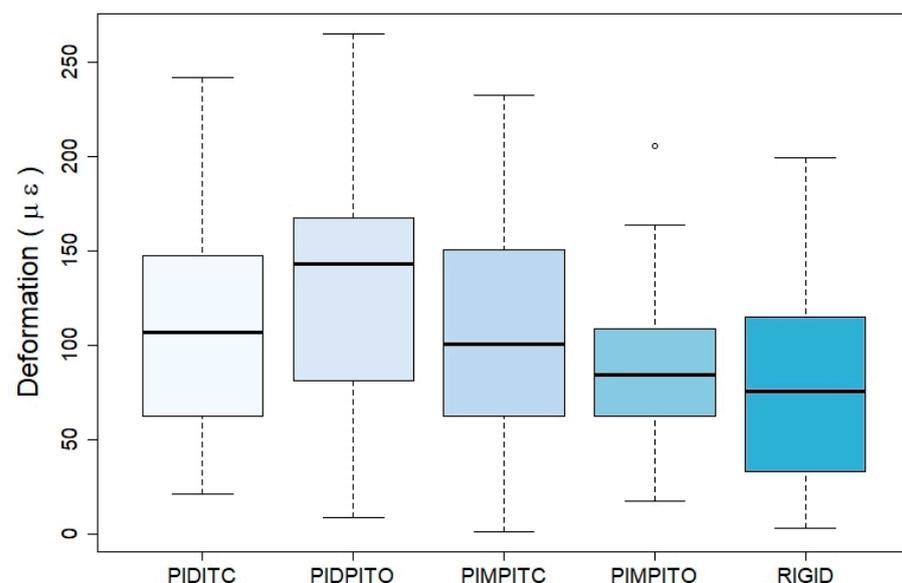
**Figure 13.** Boxplot of principal strains by bridge models.
