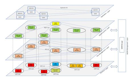
Figure 1. EQUO QKDN functional architecture.
