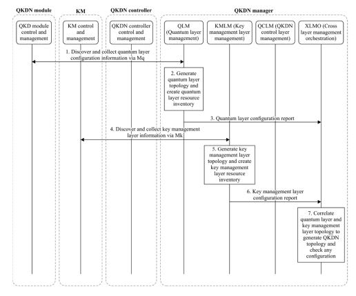
Figure 7. QKDN topology discovery procedure (source: ITU-T Y.3804).
