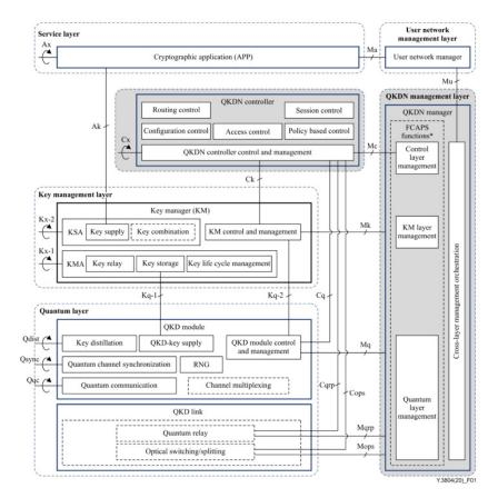
**Figure 2.** Functional elements and reference points relevant to QKDN control and management (source: ITU-T Y.3804). \*: Traditional fault, configuration, accounting, performance, and security (FCAPS) functionality which is not specific to QKDN is outside the scope of this Recommendation.
