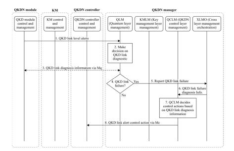
Figure 5. QKD link failure procedure (source: ITU-T Y.3804).
