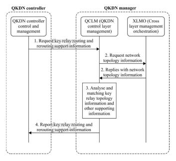
Figure 4. Key relay rerouting procedure (source: ITU-T Y.3804).
