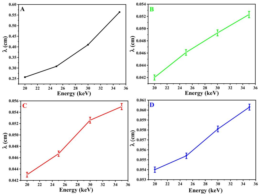
Figure 15. The dependence of the mean free path (15) on the energy of epoxy and nanocomposites at a range of operating voltages.
