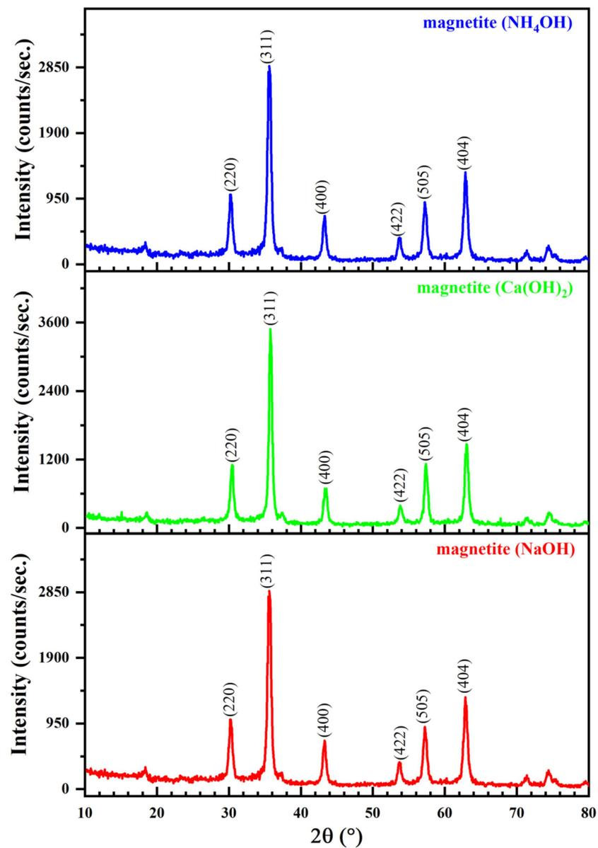
**Figure 1.** Transmitted intensity of the X-ray diffraction (XRD) patterns as a function of Bragg's diffraction angle of magnetite NPs with different sedimentation rules. The values in the parentheses represent (*hkl*) planes.
