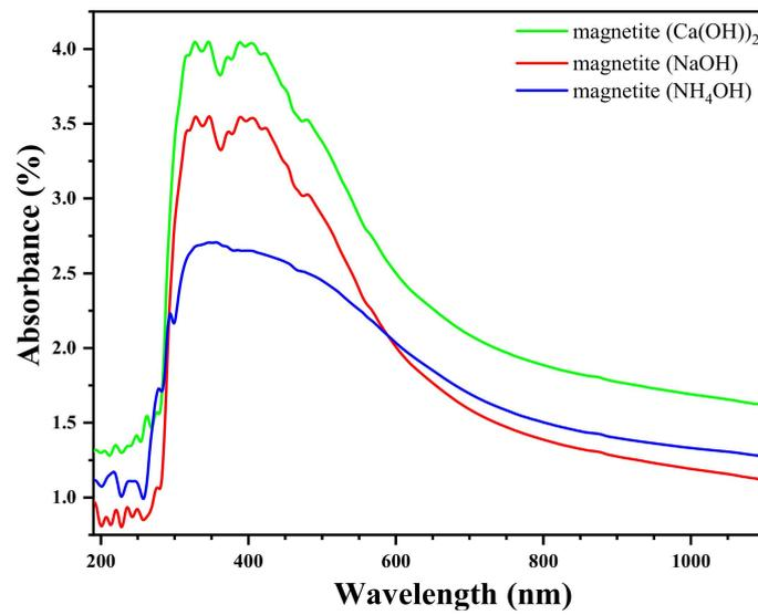
Figure 7. Ultra-violet UV-visible absorption spectra of magnetite NPs with different sedimentation rules.
