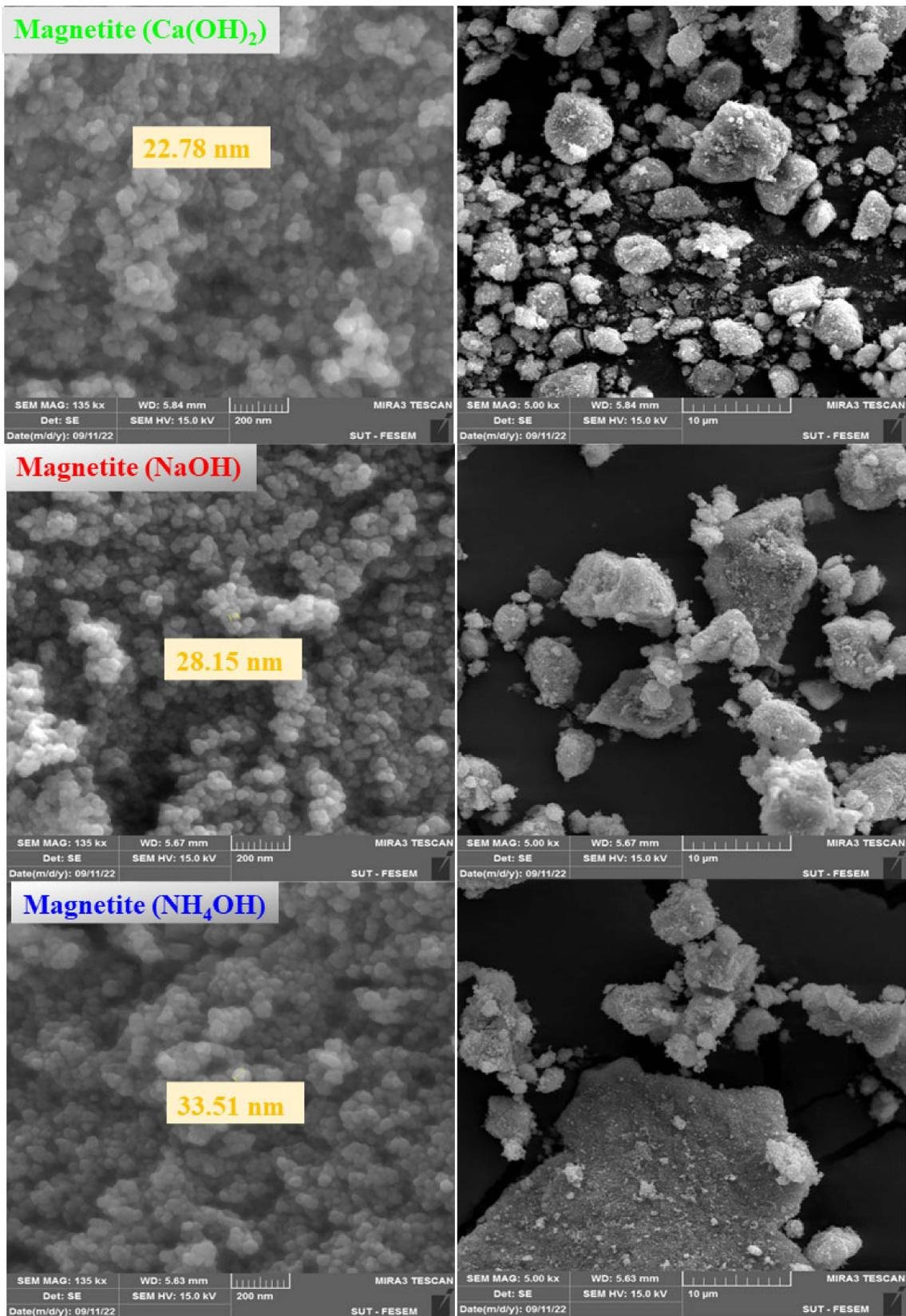
**Figure 3.** The scanning electron microscopy (SEM) images, with the nanoparticle size indicated, at 200 nm (left) and 10 μm (right) resolutions of magnetite NPs with different sedimentation rules.
