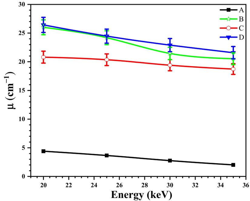
Figure 12. The dependence of the linear attenuation coefficient (12) on the energy of epoxy and nanocomposites at a range of operating voltages.
