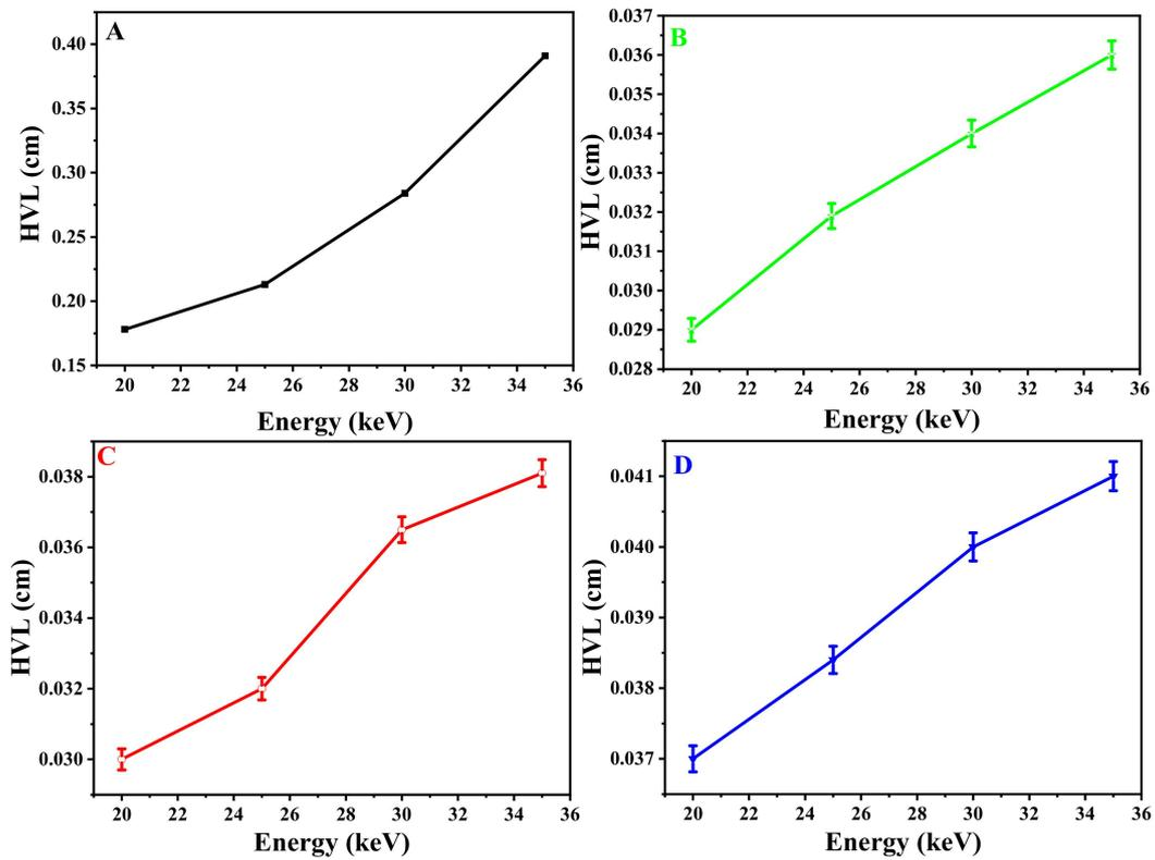
Figure 14. The dependence of the half-value layer (14) on the energy of epoxy and nanocomposites at a range of operating voltages.
