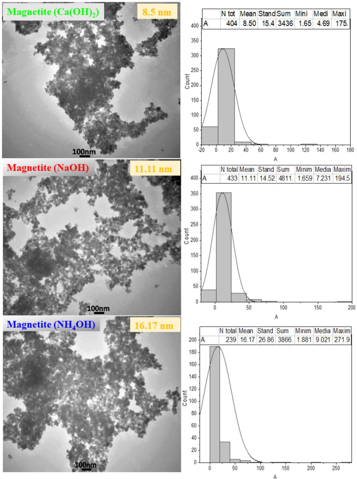
**Figure 2.** The transmission electron microscopy (TEM) images (left) with the measured nanoparticle size indicated and the nanoparticle size distribution histograms (right) of magnetite NPs with different sedimentation rules.
