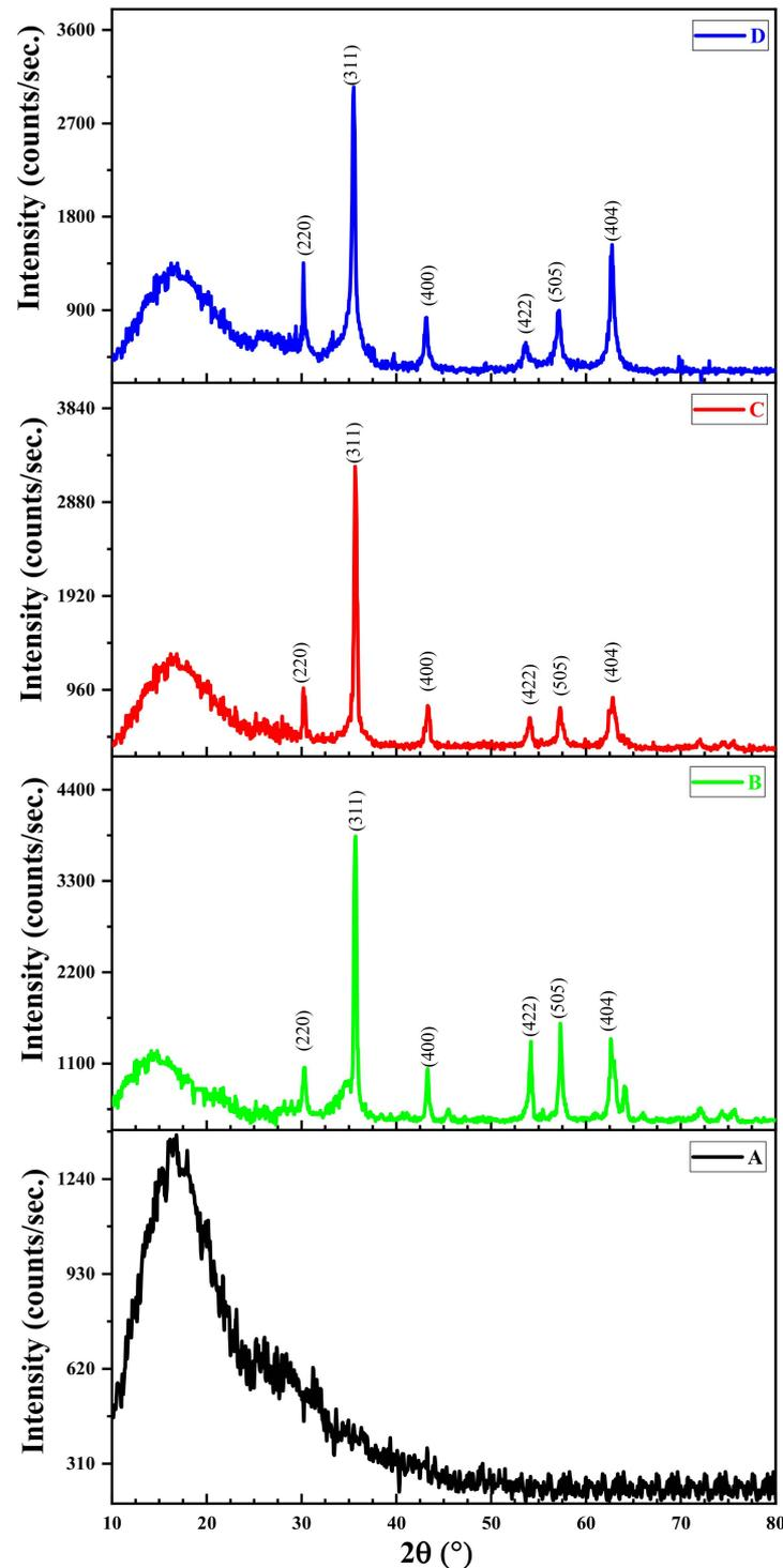
**Figure 9.** The XRD patterns of the intensity dependence on the Bragg's angle of epoxy and nanocomposites. The values in the parentheses represent  $(hkl)$  planes.
