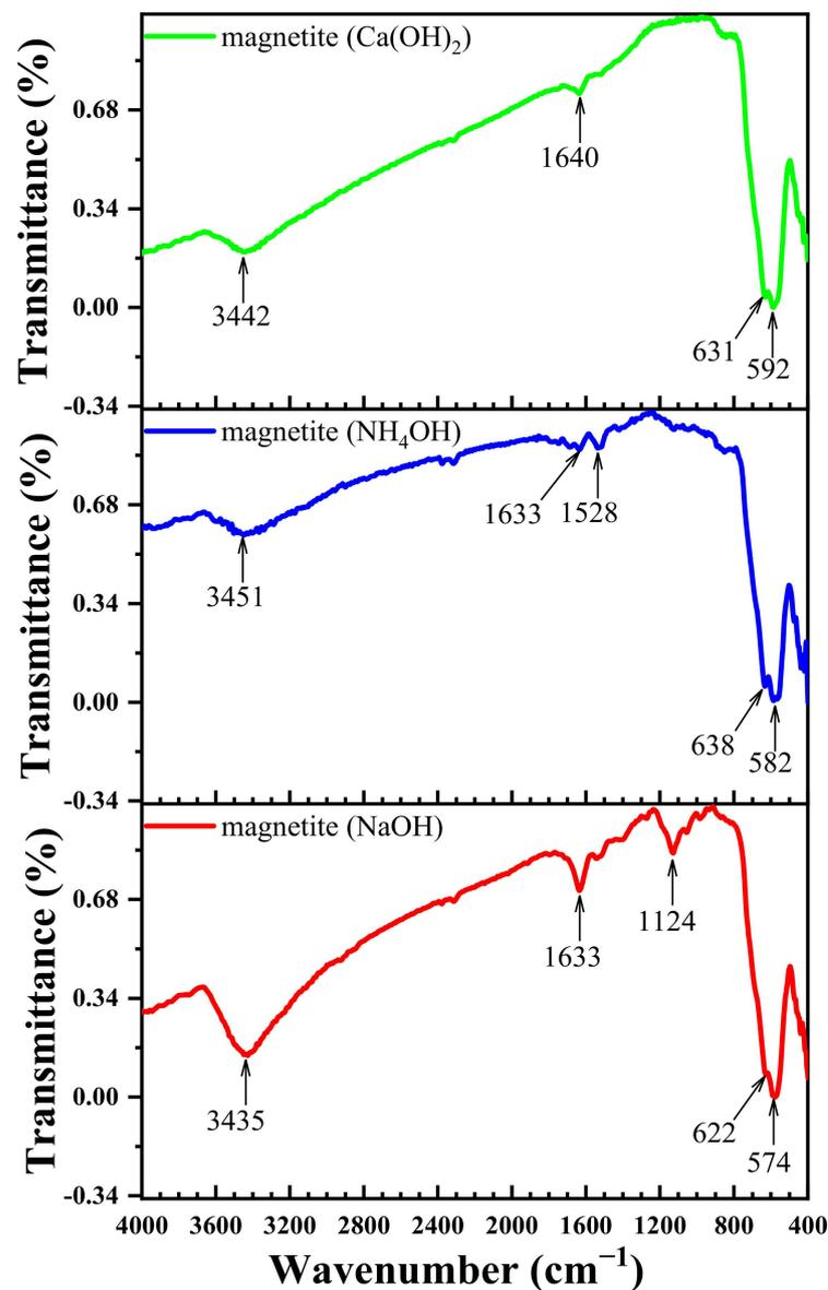
**Figure 6.** The Fourier-transformed infrared (FT-IR) spectra of magnetite NPs with different sedimentation rules.
