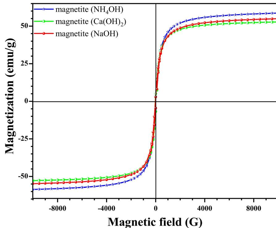
**Figure 5.** The magnetic hysteresis ring of magnetite NPs with different sedimentation rules.
