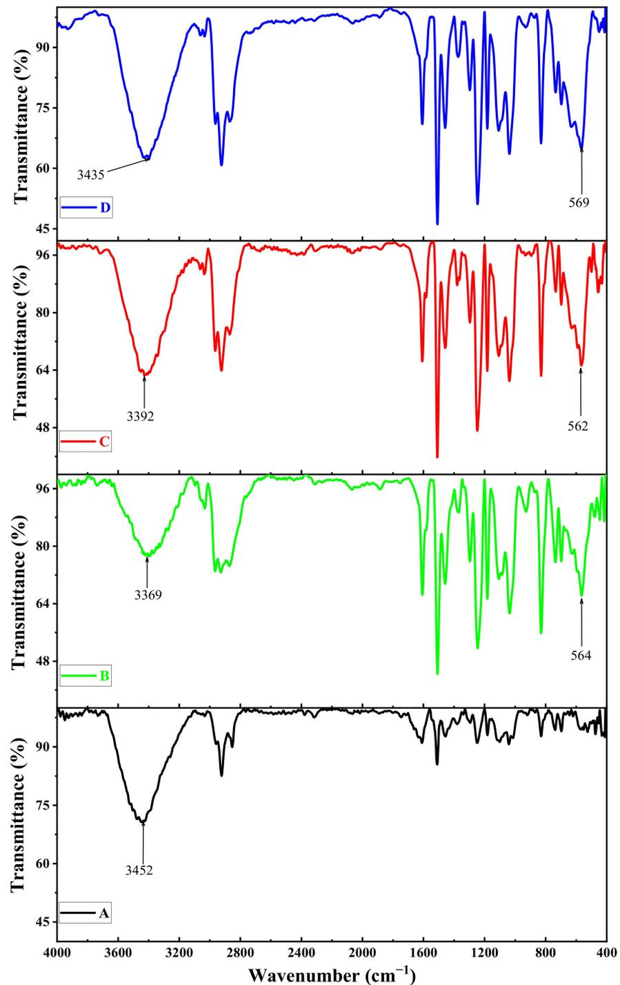
**Figure 11.** The FT-IR spectra of epoxy and nanocomposites.
