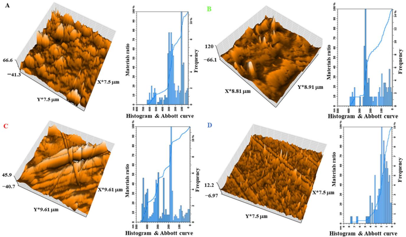
Figure 10. Atomic force microscope images of epoxy and nanocomposites.
