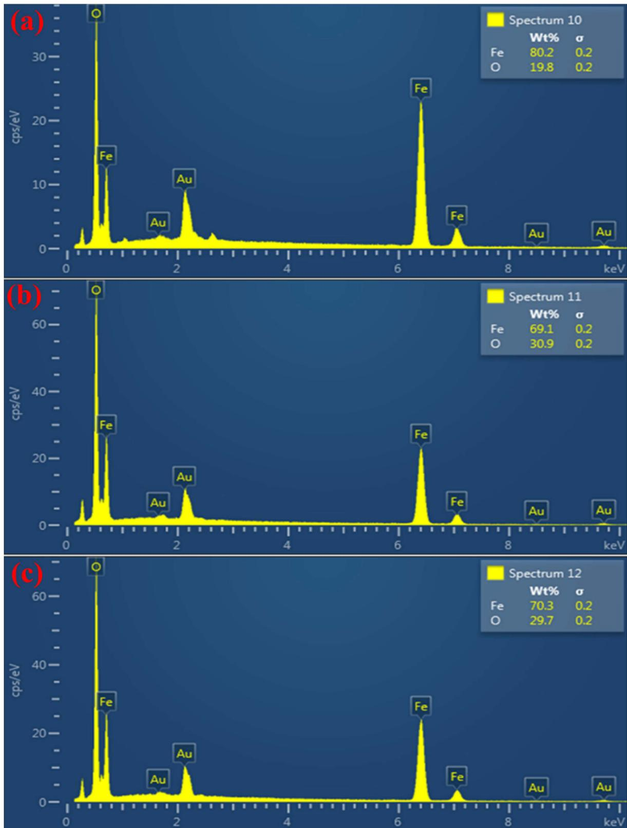
**Figure 4.** The energy-dispersive X-ray (EDX) analysis spectra of magnetite NPs prepared using (a) Ca(OH)<sub>2</sub>, (b) NaOH, and (c) NH<sub>4</sub>OH.
