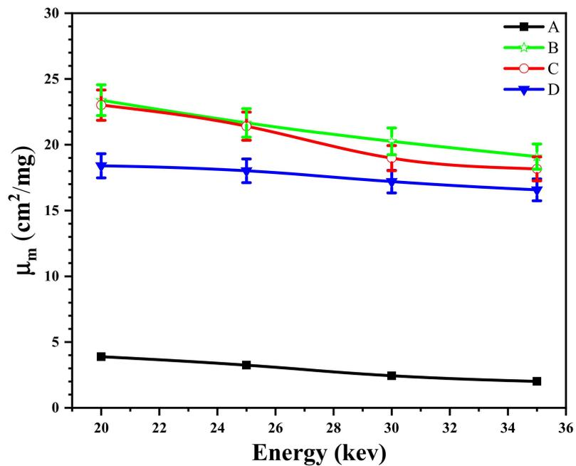
Figure 13. The dependence of the mass attenuation coefficient (13) on the energy of epoxy and nanocomposites at a range of operating voltages.
