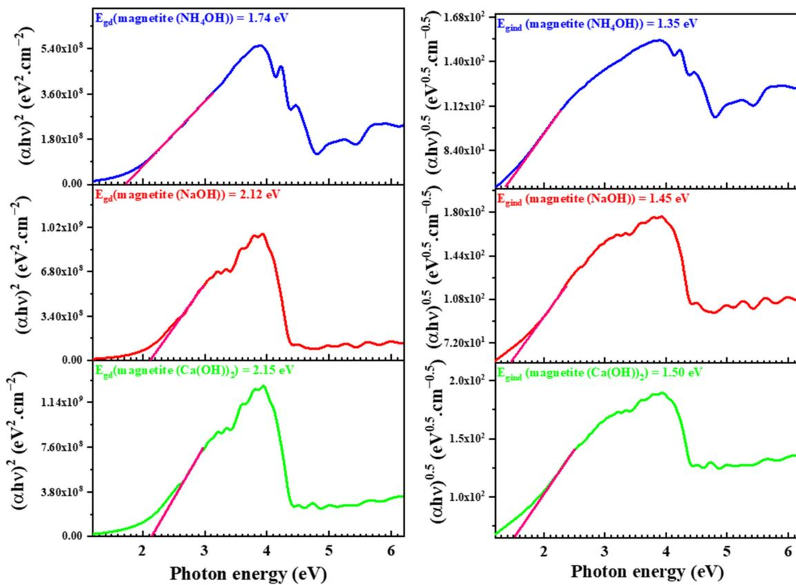
Figure 8. The allowed direct and indirect transitions (see Equation (11)) of magnetite NPs with different sedimentation rules. Here,  $E_{gd}$  and  $E_{gind}$  denotes the direct and indirect energy gap ( $E_g$ ), respectively.
