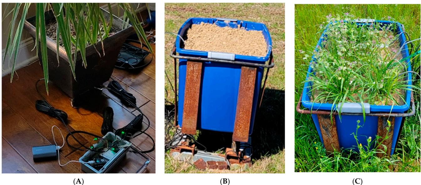
**Figure 6.** Experimental setup for the indoor and outdoor experiments. (A) Flowerpot with four load cells underneath. (B) Soil container with four load cells underneath. (C) Soil container with weeds.
