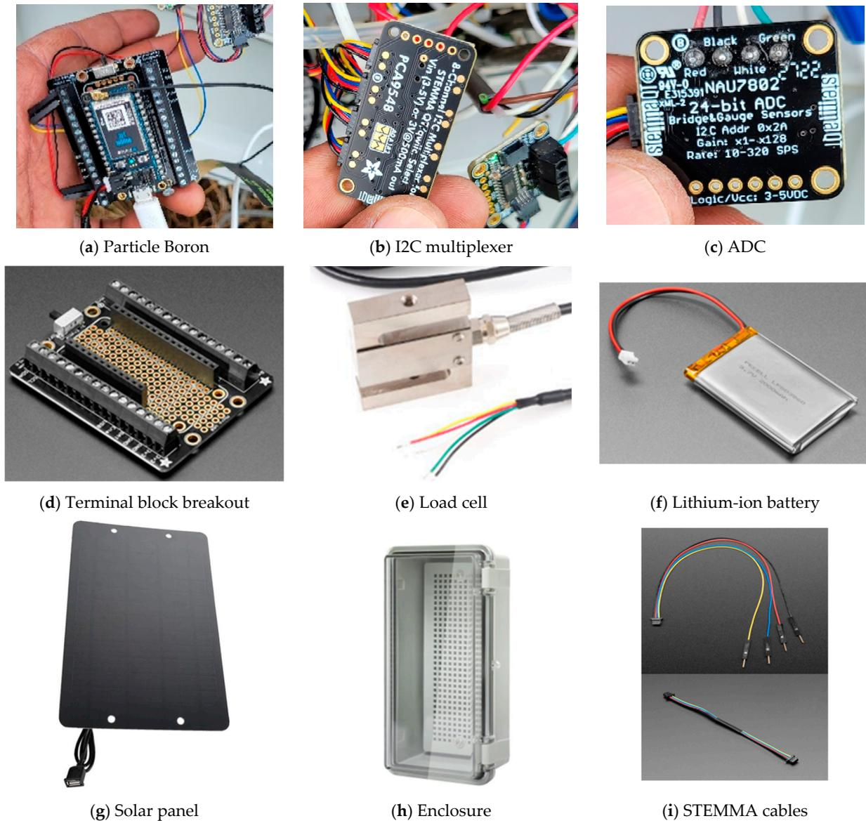
**Figure 3.** Electronic components for IoT scale system.
