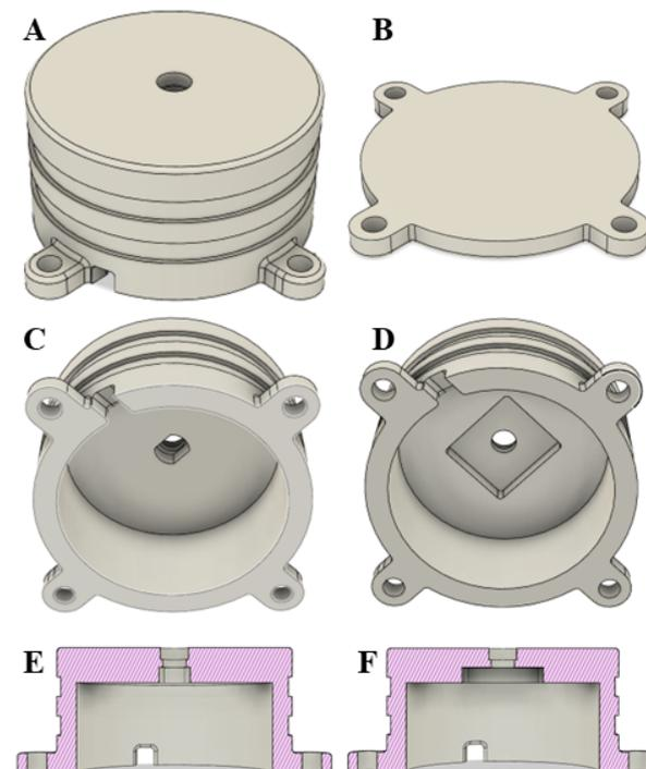
Figure 3. Enclosure design. (A): Outside of the enclosure. (B): Bottom plate of the enclosure. (C): Inside of the enclosure for the photodiode. (D): Inside of the enclosure for SI 1145. (E): Cross-section of enclosure for the photodiode. (F): Cross-section of enclosure for the SI 1145.
