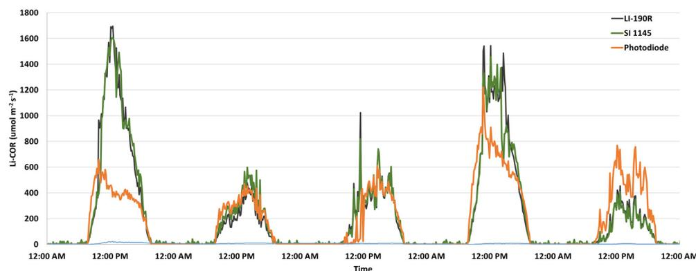
**Figure 10.** Comparison of LI-190R, SI 1145, and photodiode in outdoor environment conditions.
