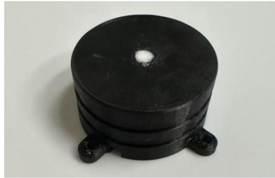
**Figure 4.** 3D-printed housing for SI 1145 and photodiode.
