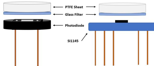
Figure 2. Diagram of the layout of the PTFE sheet and glass filter for the photodiode and SI1145.
