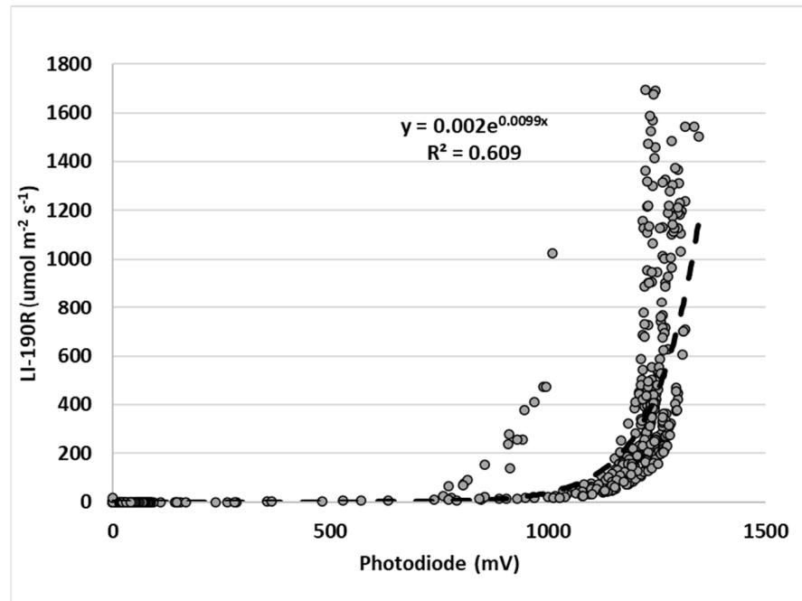
Figure 8. Comparison of photodiode with LI-190R from the calibration process.
