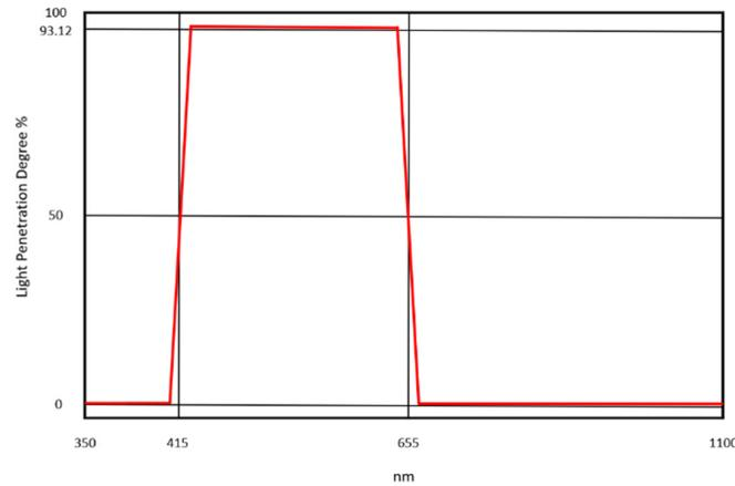
Figure 1. Light penetration of the UV AR IR glass-cut filter.
