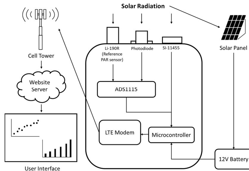
**Figure 5.** System diagram of the IoT-based PAR sensor monitoring system.
