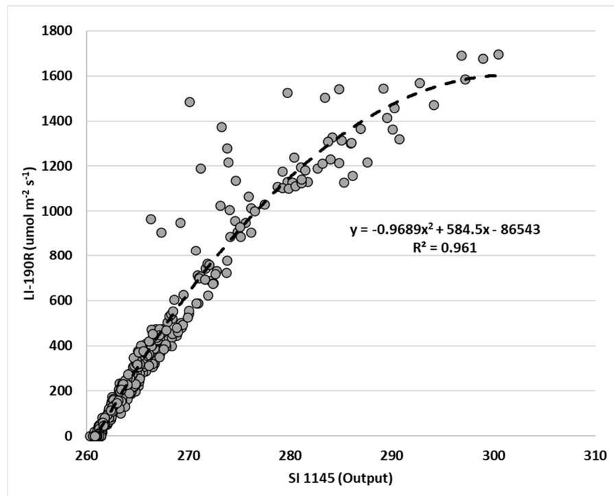
Figure 9. Comparison of SI 1145 with LI-190R from the calibration process.
