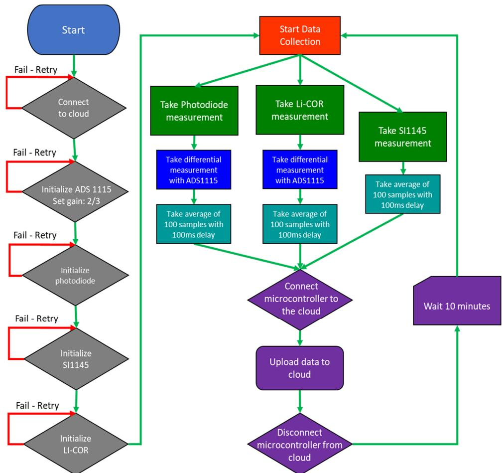
Figure 7. Flow of the microcontroller program.
