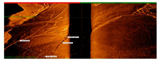
**Figure 22.** The widest section of the Lixi waterways varies between 110 m and 136 m wide, with their original depths fluctuating from 5 m to 6 m. GPS coordinates: 23°50.89608' N, 114°27.93038' E, with a current depth of 27.5 m.
