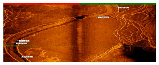
**Figure 14.** Tributaries of Nanhu waterways, with varying widths of 16.674 m to 23 m and original depths of 3.3 m to 12 m. GPS coordinates: 23°47.99988' N, 114°36.65348' E.
