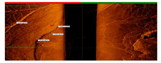
**Figure 21.** The old Huilong channel is 179 m wide, with its original depths varying between 18 m and 21 m. GPS coordinates: 23°46.09602' N, 114°30.70368' E, with a current depth of 41.7 m.
