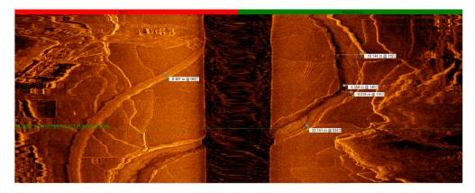
**Figure 13.** The highway near the Nanhu waterways spanned a width of 8.5 m. The waterways varied in width, ranging from 9.0 m to 22.151 m, with a depth of 4.3 m. GPS coordinates:  $23^{\circ}48.33232'$  N,  $114^{\circ}37.11502'$  E.
