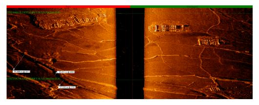
**Figure 23.** The narrowest section of the Lixi waterways ranges from 27 m to 65 m in width, with a depth of 19 m. GPS coordinates: 23°50.31488' N, 114°26.91404' E, with a current depth of 23.1 m.
