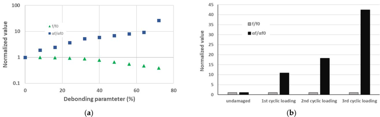
**Figure 37.** Nonlinear elastic parameter sensibility against the linear frequency loss parameter: debonding on sandwich (a) (adapted from [67]) and fatigue damage induced on laminate (b) (adapted from [66]).
