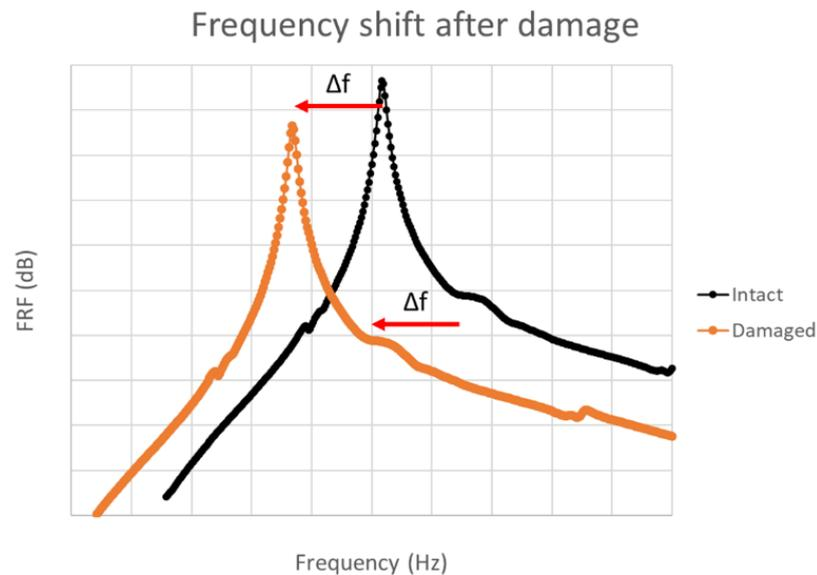
Figure 10. Natural frequency shift induced by damage.
