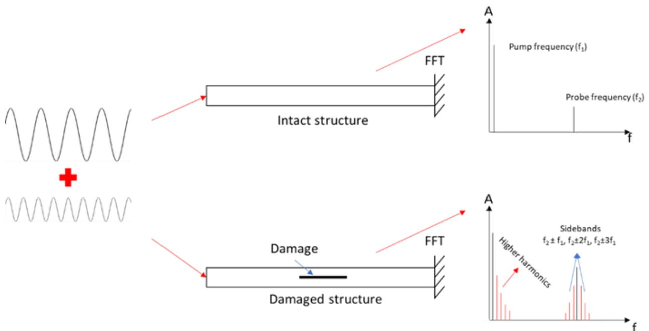
**Figure 40.** Schematic of the VAM method (adapted from [120]).
