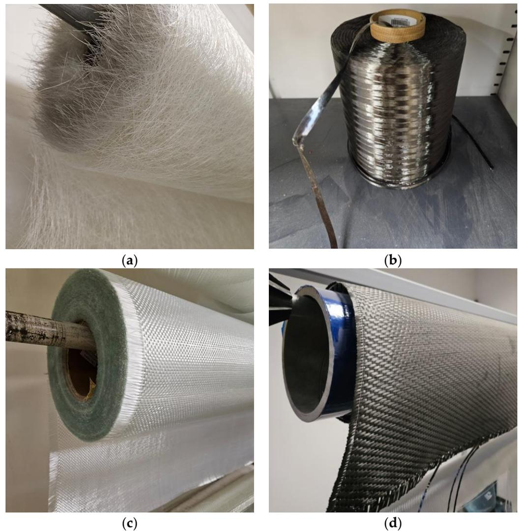
**Figure 3.** Different architectures of fibers: (a) mat short glass fiber, (b) continuous carbon fiber, (c) plain glass fiber, and (d) twill 2/1 carbon fiber.
