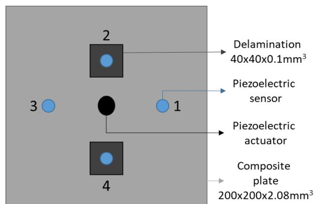
**Figure 32.** Composite plate with 5 PZT transducers and 2 delaminations (adapted from [120]).
