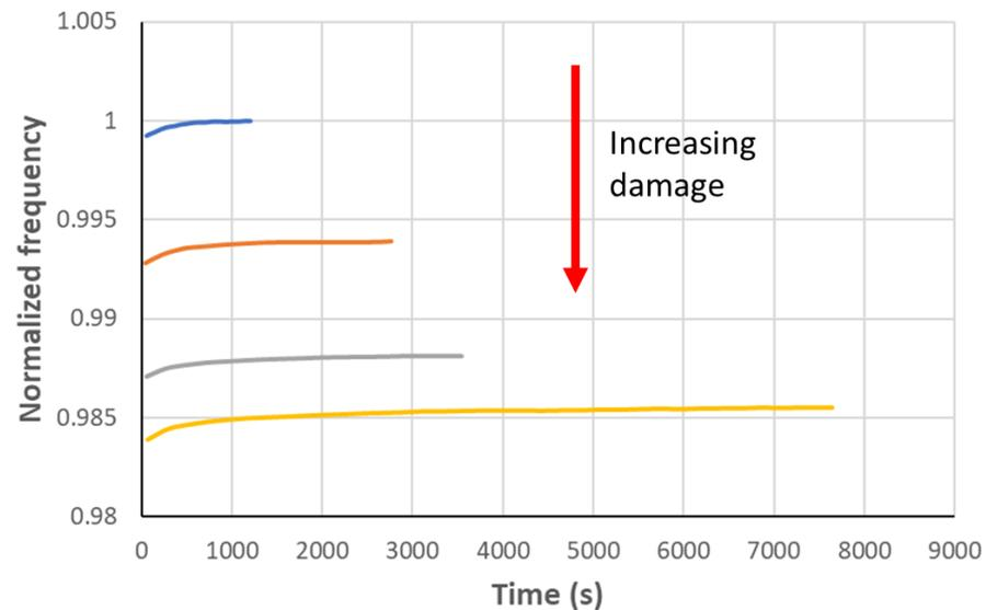
Figure 39. Time of relaxation of 4 damage levels of a PMC structure (adapted from [131]).
