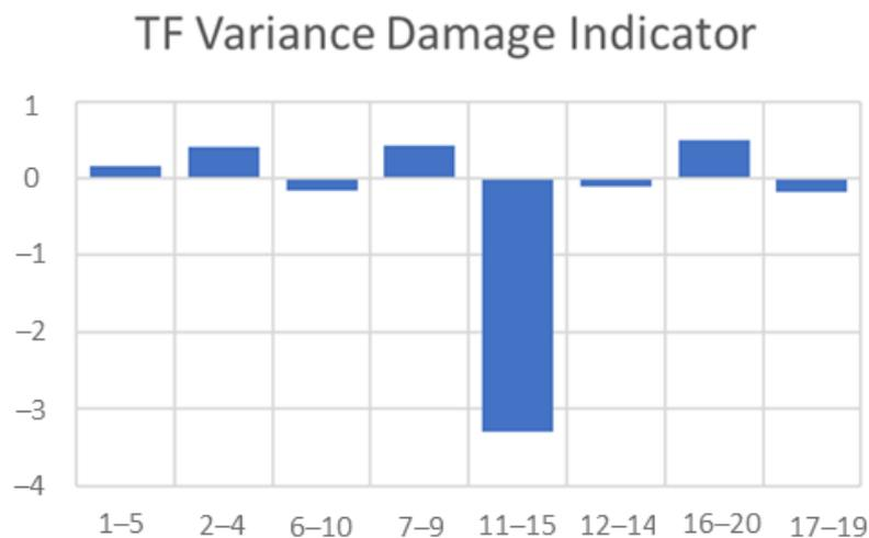
**Figure 28.** TF variance DI, damage between path 11–15 (adapted from [116]).
