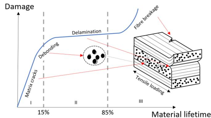
**Figure 5.** Evolution of damage in composite laminate (adapted from [40]).
