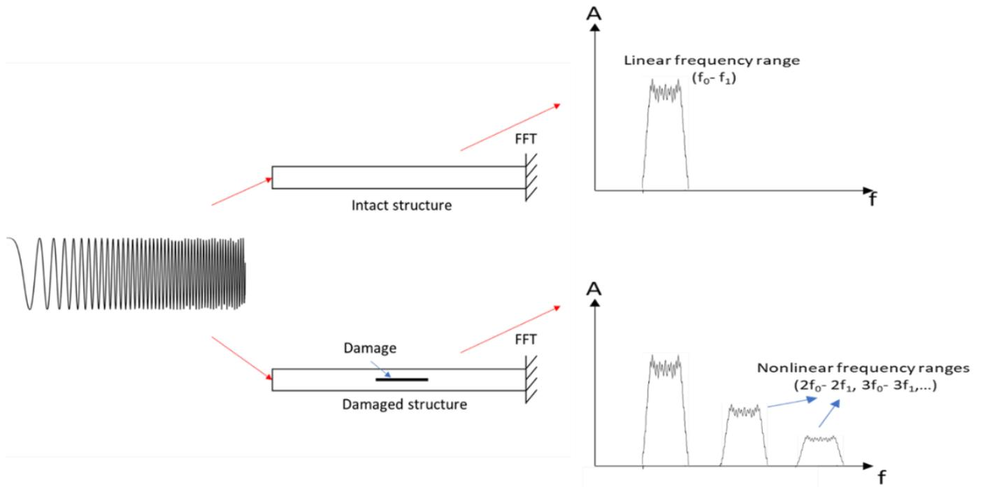
Figure 35. Schematic of the SWP method (adapted from [120]).
