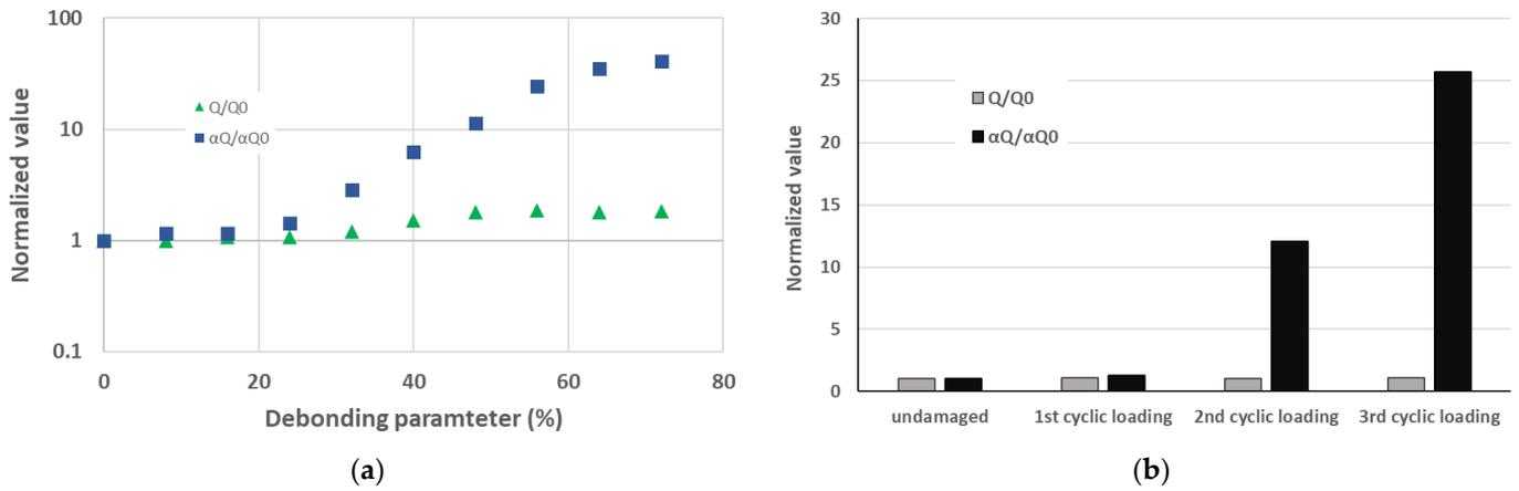
**Figure 42.** Nonlinear dissipative parameter sensibility against the linear loss factor parameter: debonding on a sandwich (a) (adapted from [67]) and fatigue damage induced on the laminate (b) (adapted from [66]).
