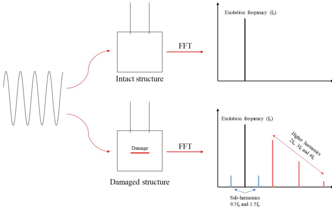
Figure 29. Schematic of the SFE method (adapted from [120]).
