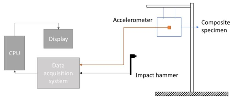
**Figure 15.** Schematic of the experimental setup (adapted from [79]).
