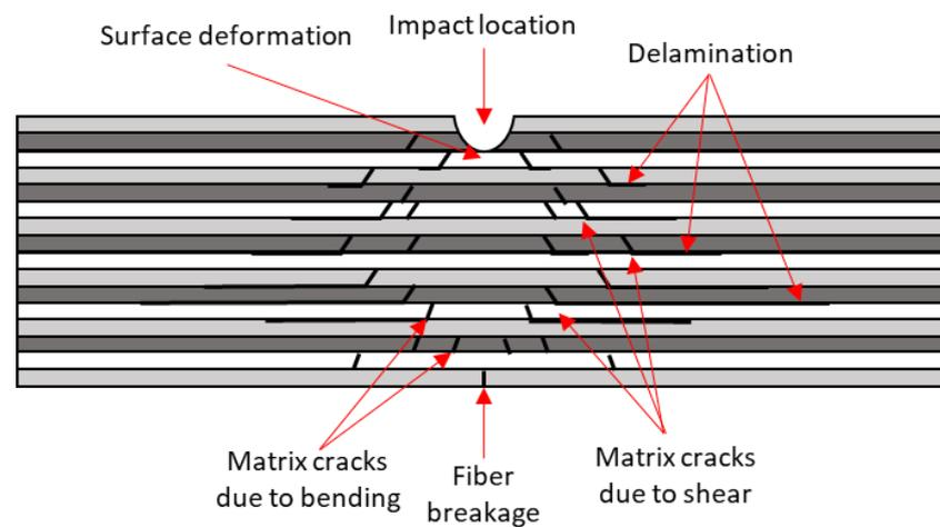
**Figure 4.** Impact damage mechanisms in composite laminate (adapted from [39]).
