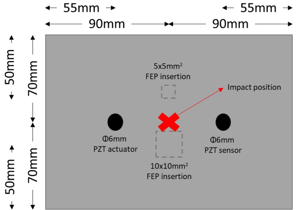
Figure 34. Specimen and damage specification (adapted from [123]).
