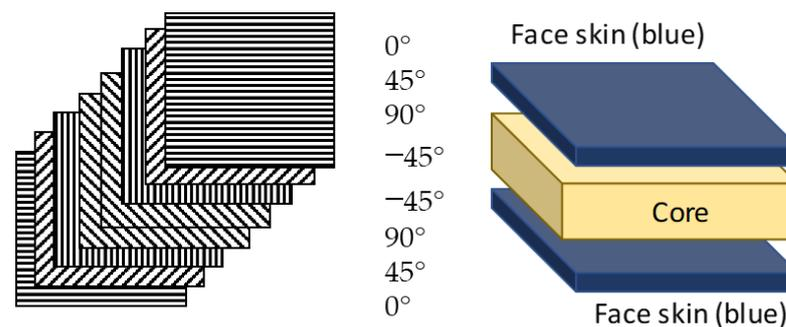
**Figure 2.** Laminated (left) and sandwich composite (right).
