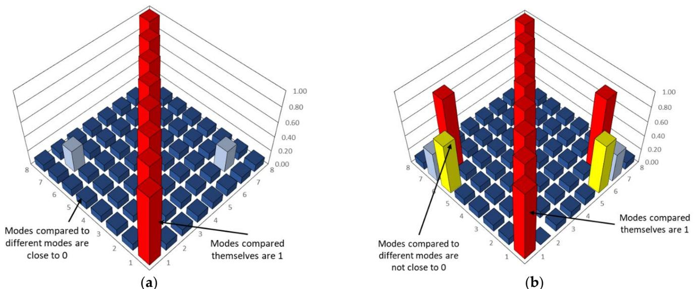
**Figure 14.** Typical MAC. No similar way of moving of the modes (a) and some modes with a similar way of moving (b).
