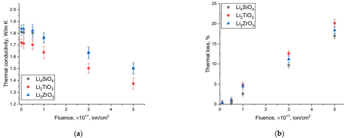
**Figure 6.** The results of changes in the thermophysical parameters of the ceramics under study as a function of the irradiation fluence: (a) change in the thermal conductivity coefficient of the ceramics; (b) change in heat losses (deterioration of thermal conductivity coefficient).
