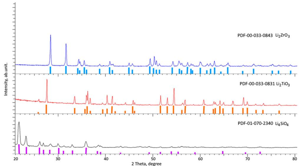
**Figure 1.** X-ray diffraction patterns of the studied  $\text{Li}_4\text{SiO}_4$ ,  $\text{Li}_2\text{TiO}_3$ , and  $\text{Li}_2\text{ZrO}_3$  ceramics in the initial state, obtained using the mechanochemical synthesis method.
