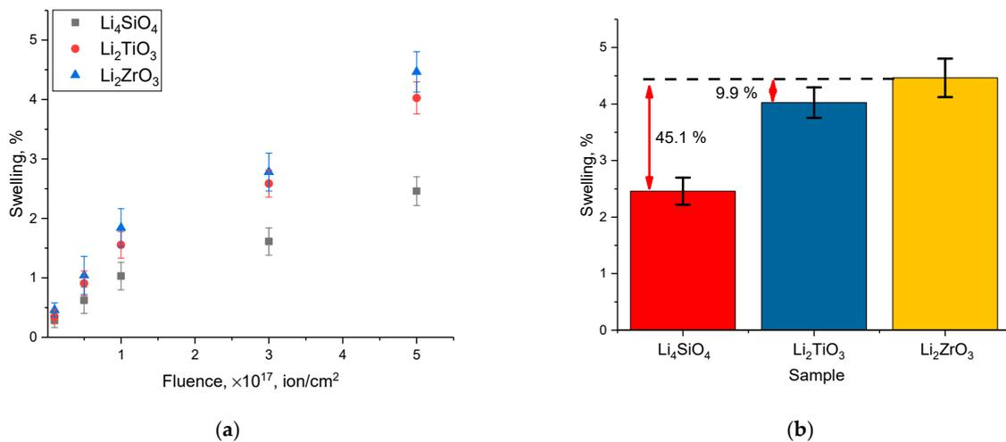
**Figure 4.** (a) The assessment results of the crystal lattice swelling value as a function of the irradiation fluence of lithium-containing ceramics; (b) the results of a comparative analysis of the maximum swelling value of ceramics at an irradiation fluence of  $5 \times 10^{17}$  ions/cm<sup>2</sup> (arrows indicate the difference in swelling of  $\text{Li}_4\text{SiO}_4$  and  $\text{Li}_2\text{TiO}_3$  ceramics in comparison with  $\text{Li}_2\text{ZrO}_3$  ceramics).
