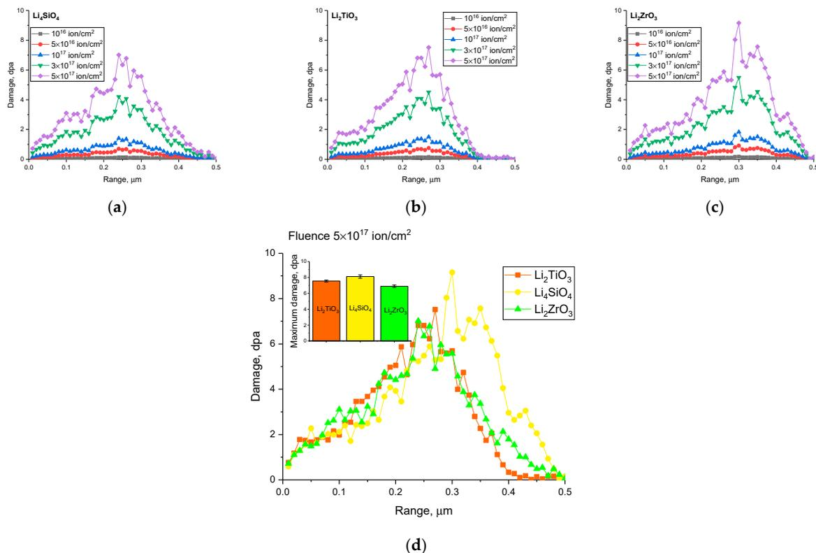
**Figure 3.** The assessment results of the value of atomic displacements along the trajectory of ion movement in the near-surface layer of ceramics as a function of the irradiation fluence: (a) Li<sub>4</sub>SiO<sub>4</sub>; (b) Li<sub>2</sub>TiO<sub>3</sub>; (c) Li<sub>2</sub>ZrO<sub>3</sub>; (d) graph comparing the values of atomic displacements along the trajectory of movement of He<sup>2+</sup> ions in ceramics at an irradiation fluence of  $5 \times 10^{17}$  ion/cm<sup>2</sup>.
