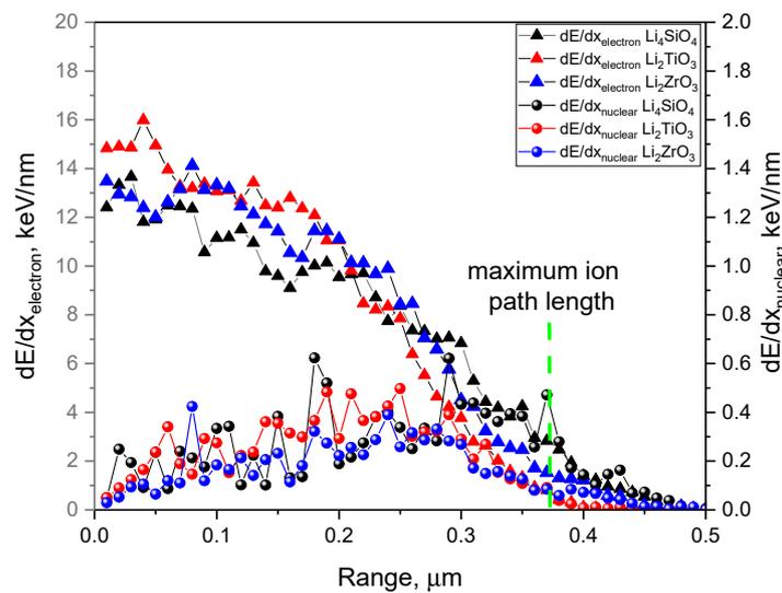
**Figure 2.** The assessment results of ionization losses of He<sup>2+</sup> ions during the interaction with the crystal structure of lithium-containing ceramics.
