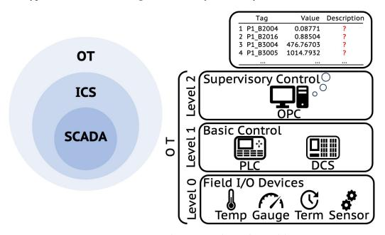
Figure 1. OT, ICS, SCADA concept map with OT part in the Purdue model.
