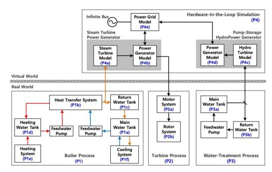
Figure 3. Hardware-in-the-loop (HIL) process flow diagram.
