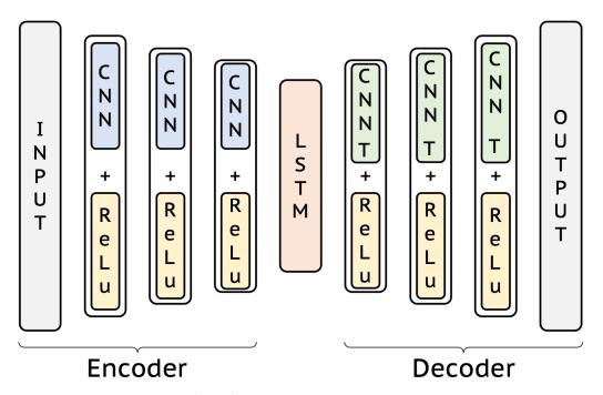
Figure 7. Composite autoencoder architecture.
