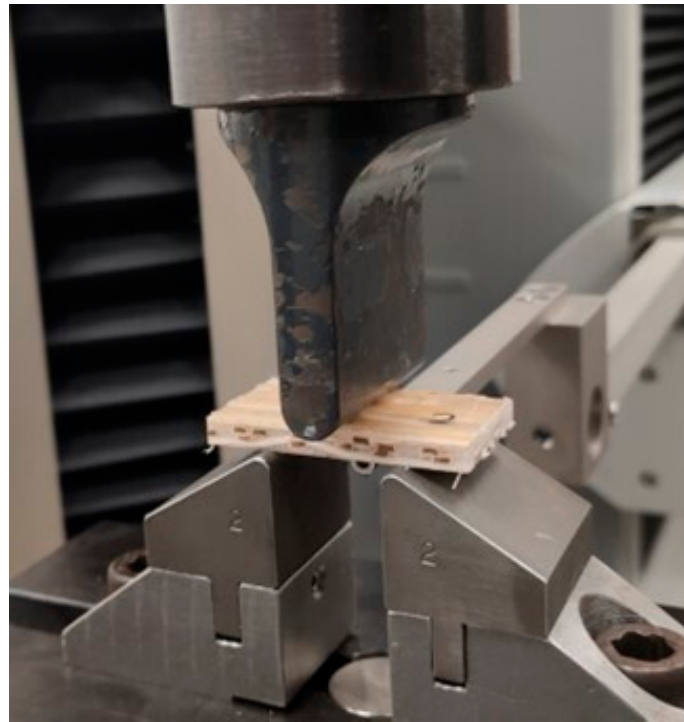
Figure 3. Set-up of the short-beam shear test.
