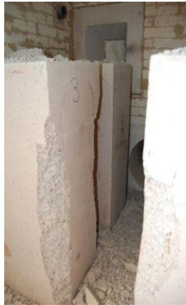
**Figure 7.** Spalling on the columns.
