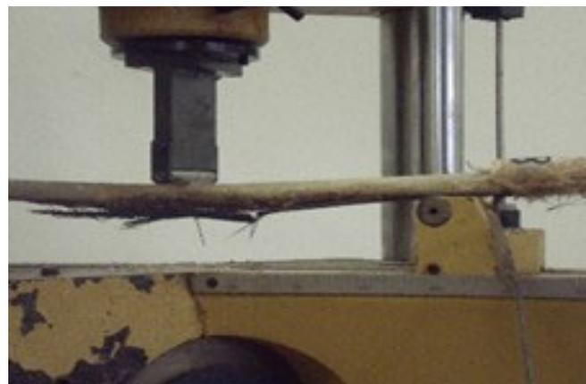
**Figure 10.** Reinforcement bending test of column 2.
