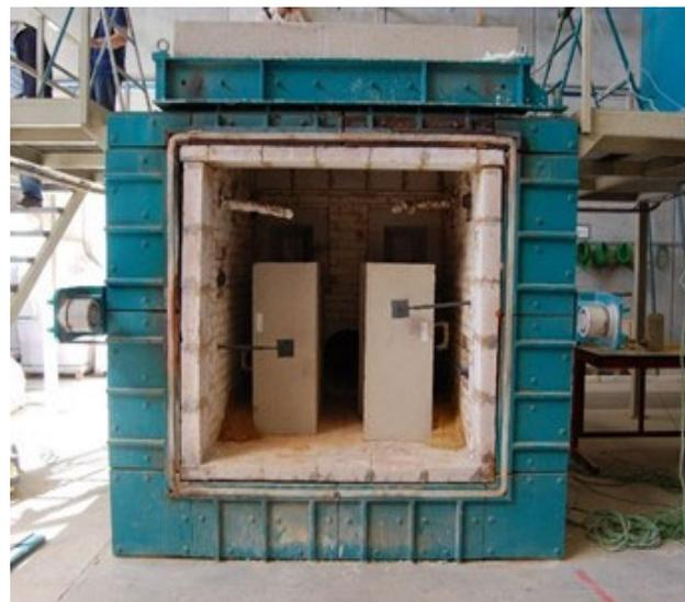
**Figure 5.** Fire test: columns placed in the furnace.
