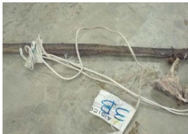
Figure 12. GFRP rebar after the fire test: column 1.
