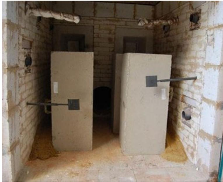
**Figure 6.** Assembly of the columns in the furnace.
