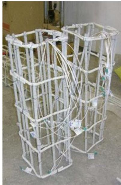
**Figure 3.** Internal column reinforcements.
