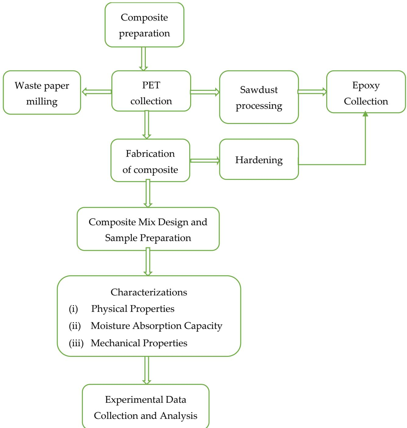
Figure 2. Process flow diagram of the composite manufacturing.
