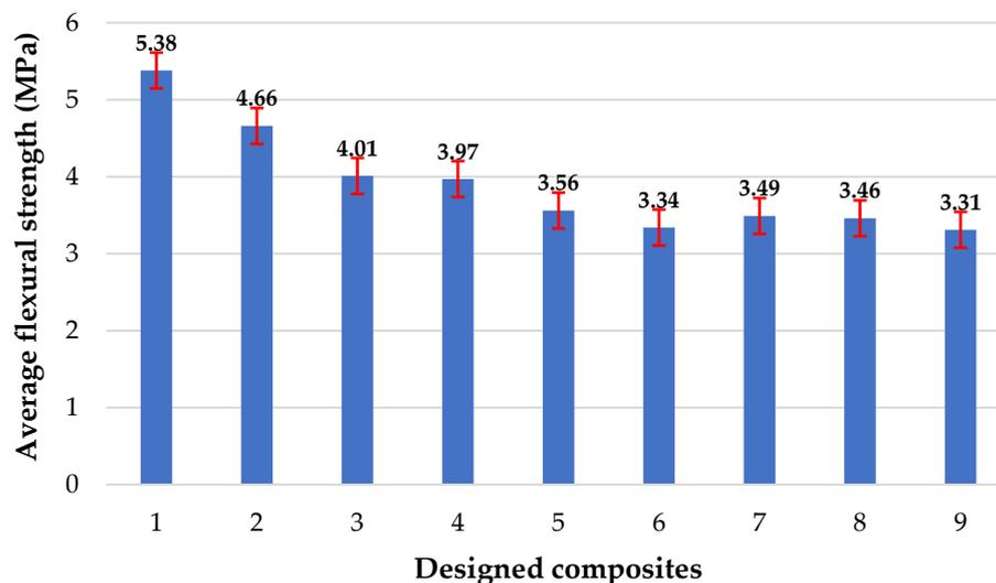
**Figure 10.** FS of the composites (MPa).
