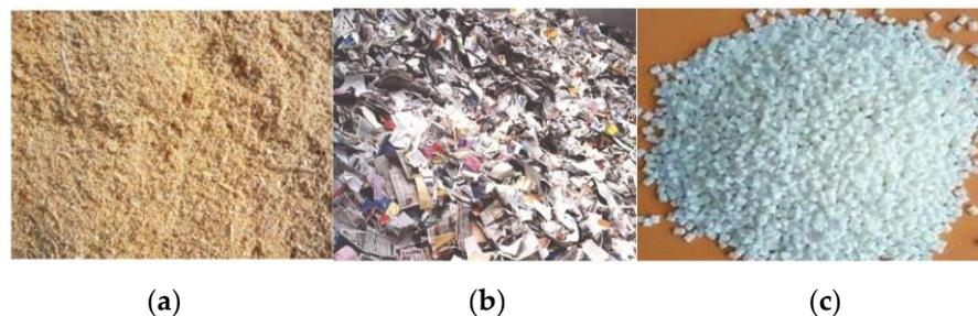
**Figure 1.** Raw materials for experimented composite manufacturing: (a) sawdust, (b) waste paper, and (c) recycled PET.
