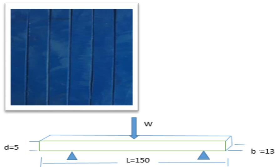
**Figure 4.** Sampling measurement of the composite board for FS.
