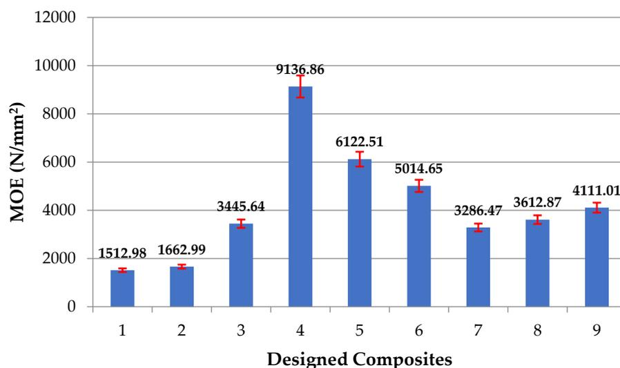
Figure 11. MOE results of experimented ceiling board composites.
