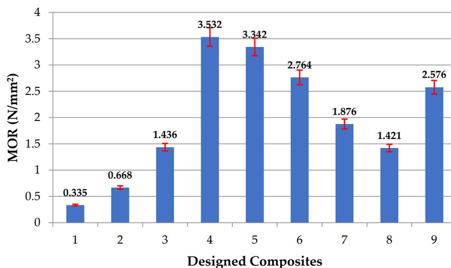
**Figure 9.** MOR results of experimented ceiling board composites.
