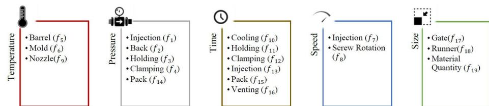
**Figure 6.** Identified features of process parameters in injection molding machine.
