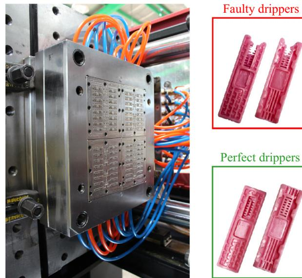
**Figure 7.** Mold of the drippers (left), faulty and perfect fabricated drippers (right).
