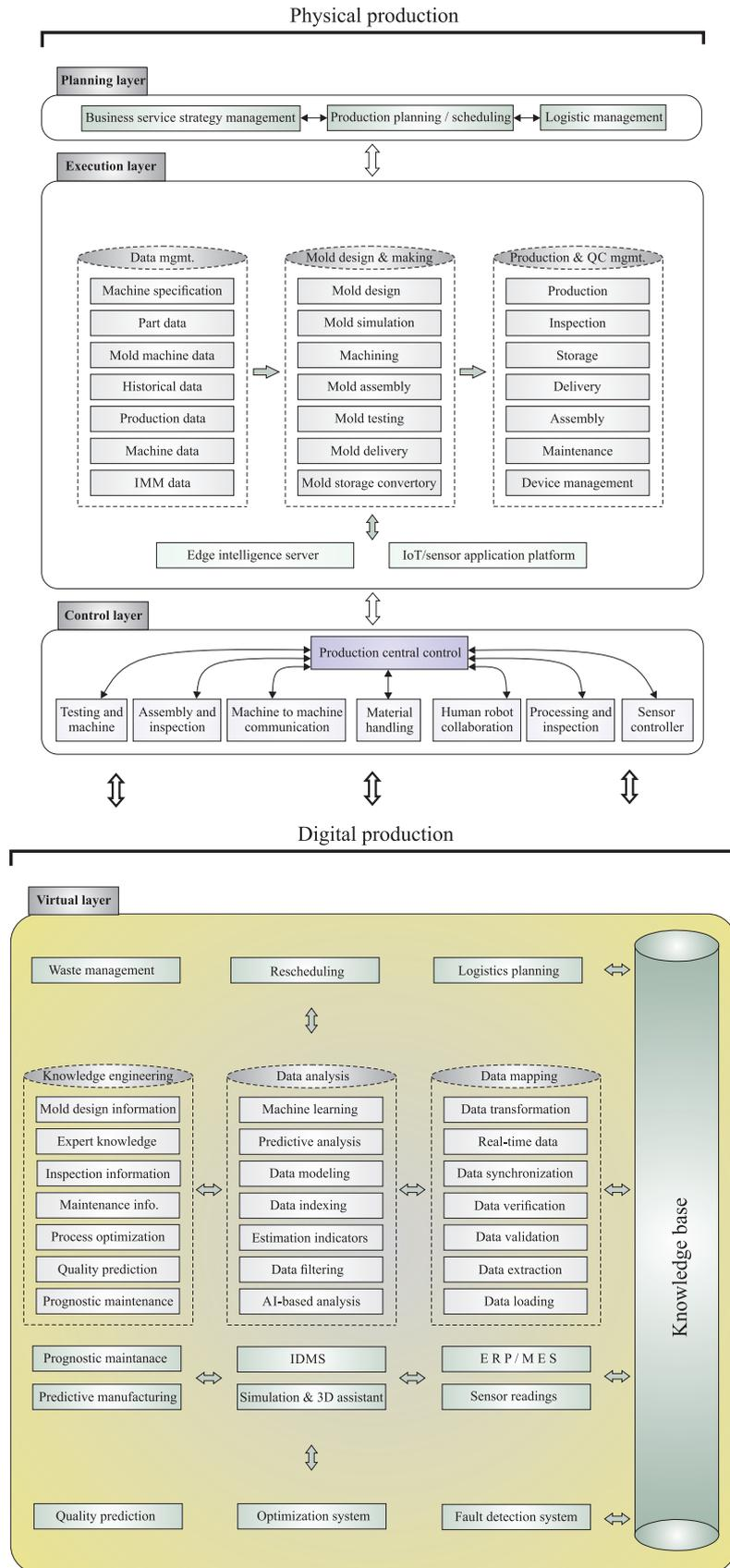
Figure 4. Knowledge-based framework of DT model for smart injection molding.
