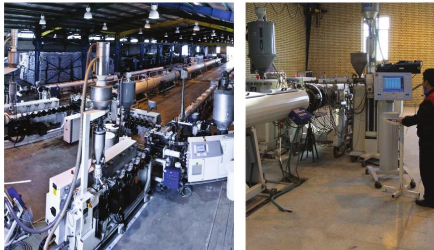
Figure 11. Injection molding and extrusion machines in Semnan Polyethylene Pipe and Fitting Co.
