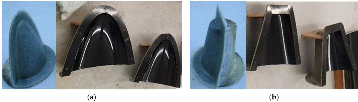
**Figure 14.** Mold and molds. (a) Front part of the fuselage. (b) Rear part of the fuselage.
