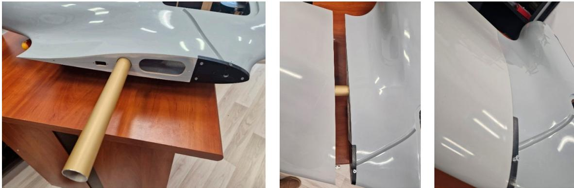
**Figure 21.** Wing–fuselage assembly.
