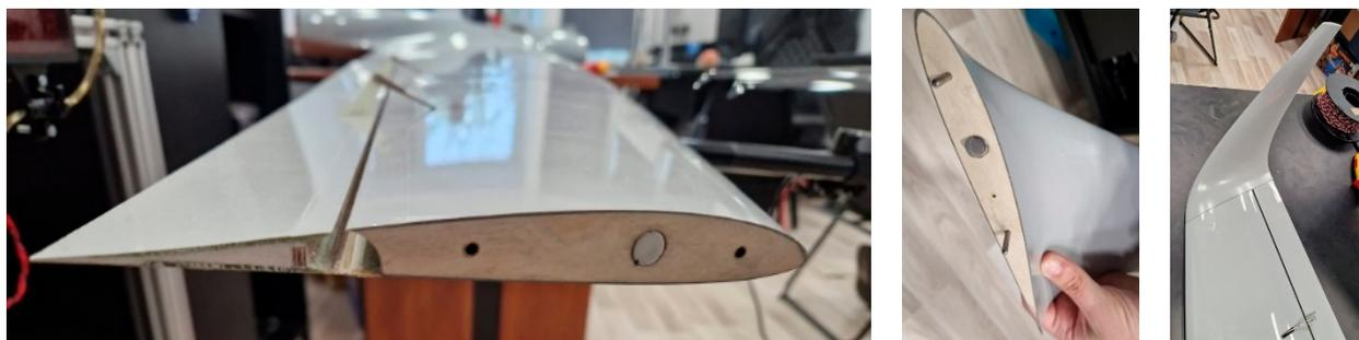
**Figure 23.** Winglet assembly—wing tip.
