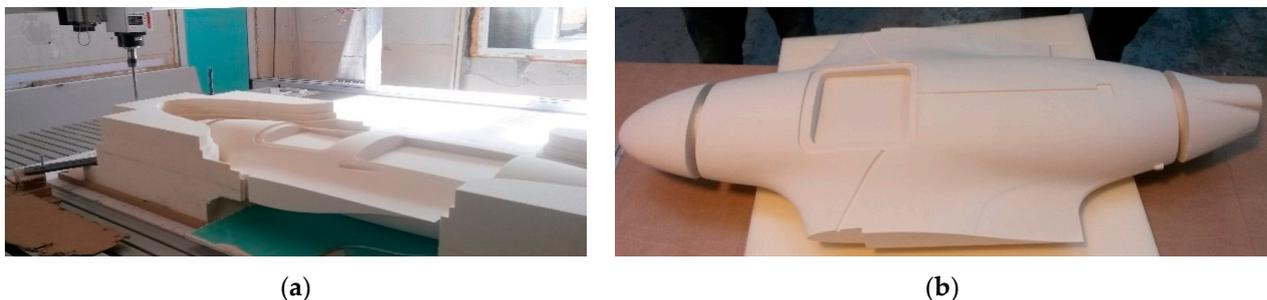
**Figure 12.** (a) Intermediary stages for the mold creation process. (b) Final molds for the aerostructure.
