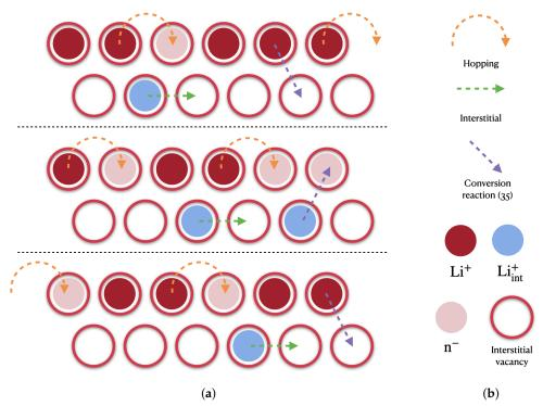
**Figure 3.** Cation migration mechanisms: hopping into uncompensated negative charges associated with vacancies in the LiPON matrix, direct interstitial and conversion after reaction (35). (a) A sequence of three ionic distribution snapshots in time; (b) Legend.
