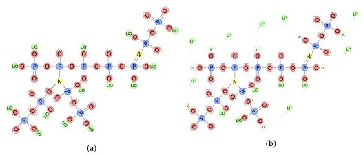
**Figure 2.** LiPON matrix contains nitrogen, which has triple and double coordination (**a**). Ionic conductivity in LiPON is achieved through the displacement of charged particles, either by hopping and vacancy-filling or by interstitial motion (**b**).
