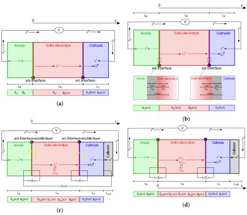
**Figure 1.** Schematics of the ASSB models proposed in the selected literature. The unknown fields, under discharge conditions, are highlighted. The yellow arrows in (c) point out the charge-transfer reactions at both interfaces. For the sake of generality, the lithium concentration in the anode is listed in the unknown fields. (a) Model in [19]; (b) model in [20]; (c) model in [21]; (d) model in [22].
