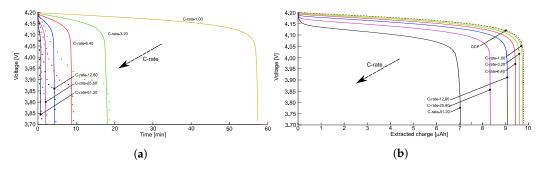
**Figure A1.** Discharge curves as a function of time (**a**), and the extracted charge (**b**) for different *C*-rates, obtained following the analytical approach to evaluate the OCP as given in [34].
