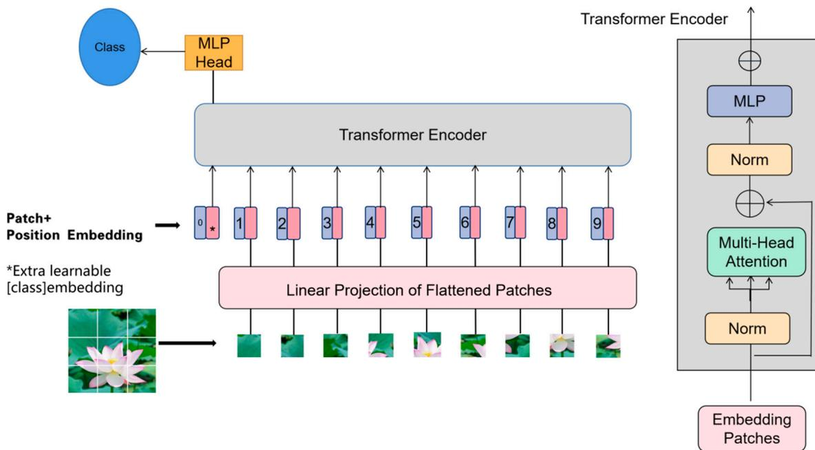
Figure 4. Schematic diagram of ViT model structure.
