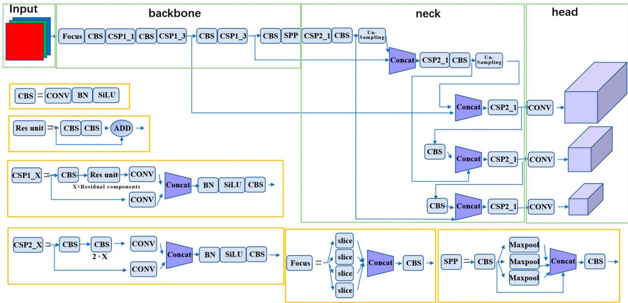
Figure 12. YOLOv5 model structure.
