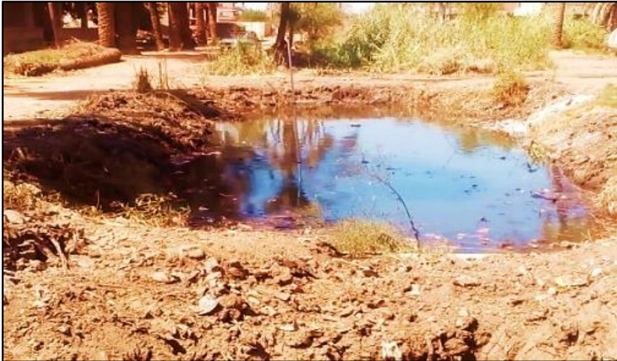
**Figure 3.** Ponding method for measuring of seepage losses.
