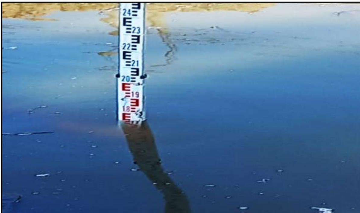
**Figure 4.** Measuring device of ponding method.
