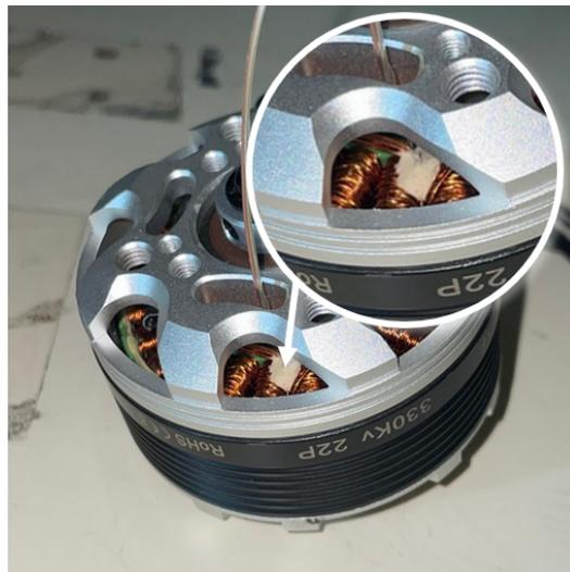
Figure 6. K-type thermocouple bonded to a motor's stator windings with thermal cement.
