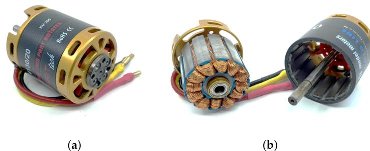
**Figure 1.** An outrunner brushless DC (BLDC) motor typically found on small UASs. (a) Fully assembled. (b) Stator (left) and rotor (right) assemblies.
