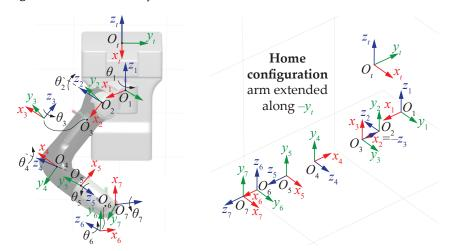
Figure 5. Reference frames of the TIAGo robotic arm.
