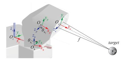
**Figure 6.** Reference frames of the TIAGo head.
