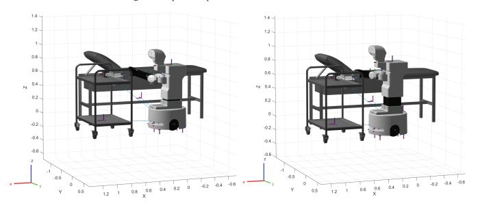
**Figure 11.** Generic posture on the left and optimized posture on the right for a given Cartesian pose where the TIAGo robot performs a grasping operation.
