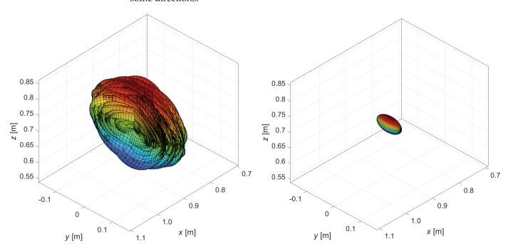
**Figure 9.** Entire set of linear velocity ellipsoids on the left and optimum velocity ellipsoid with maximum index *I* on the right.
