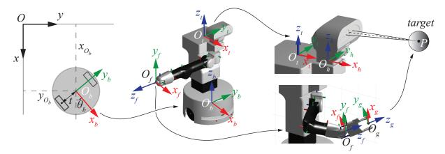
Figure 4. Main reference systems for the TIAGo robot.
