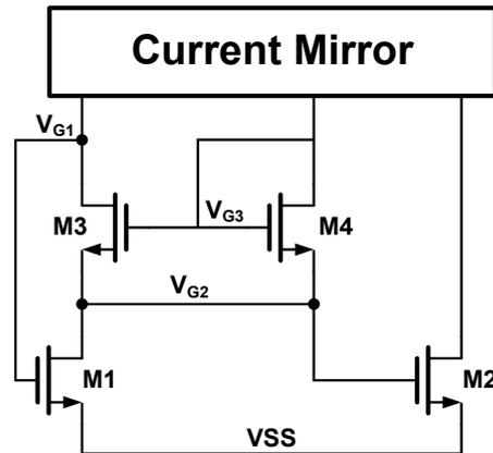
Figure 2. Core circuit of the proposed specific current source.
