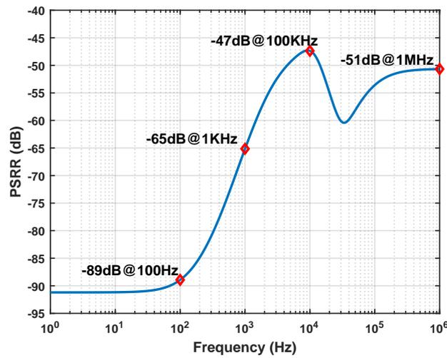
Figure 15. PSRR with a  $C_L$  of 10 pF.
