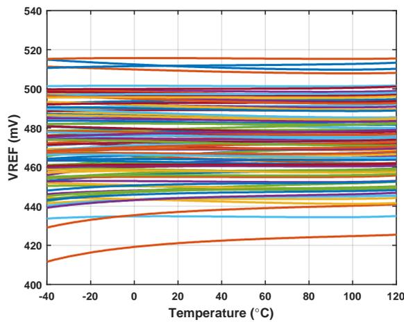
Figure 6. Monte Carlo simulation results before trimming: temperature dependence of  $V_{REF}$ .
