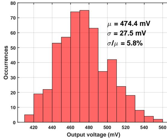
Figure 10. Histogram of average output voltage after trimming.
