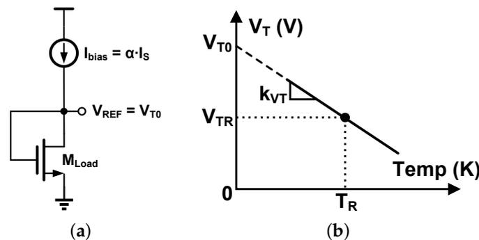
**Figure 1.** (a) The conceptual diagram of  $V_T$ -based voltage reference; (b) the temperature characteristic of  $V_T$ .
