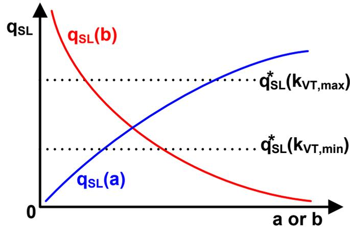
**Figure 5.** The impact of  $a$  (current mirror copy ratio) and  $b$  (size ratio  $K_L/K_4$ ) on the normalized charge density of  $M_{Load}$ .
