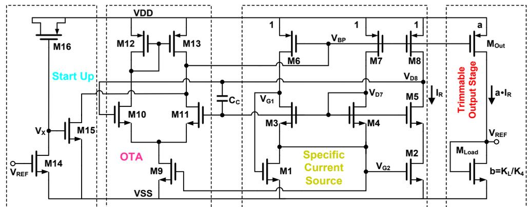
Figure 3. Schematic of the proposed  $V_T$ -based voltage reference source.
