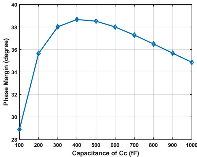
Figure 13. Phase margin as a function of  $C_C$ .
