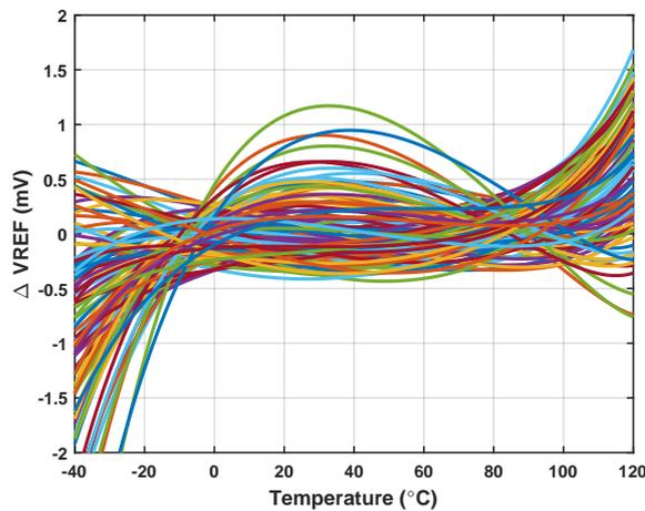
Figure 8. Monte Carlo simulation results after trimming: temperature dependence of  $\Delta V_{REF}$ .
