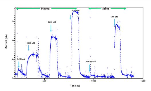
**Figure 5.** Glucose sensing in complex biological fluids. Response of biosensor to presence and absence of plasma (0.183 mM, 0.399 mM, 0.200 mM, 10.85 mM) and saliva (less than 0.111 mM and 6.44 mM).
