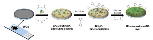
**Figure 1.** Schematic representing the steps involved in the fabrication of glucose biosensors. The sensor was constructed sequentially with a nanocomposite-based antifouling coating, surface-functionalized redox, and enzyme layers that support glucose detection in biological samples.
