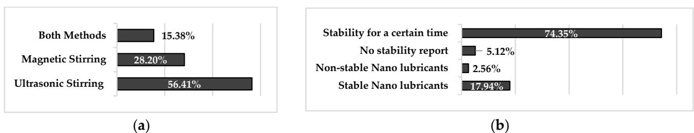
Figure 10. (a) Distribution of dispersion techniques used; (b) stability of nano-lubricants.
