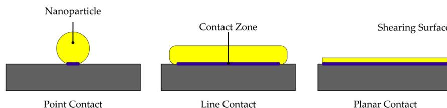
**Figure 8.** Effect of nanoparticle shape on the contact pressures experienced upon loading.
