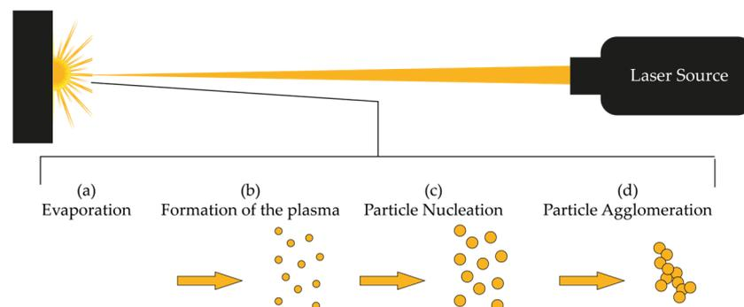
**Figure 2.** Generation of particles with the laser ablation process.
