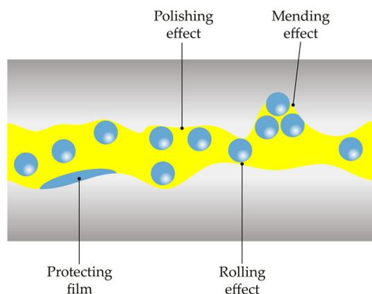
**Figure 7.** Nanoparticle lubrication mechanisms [119].
