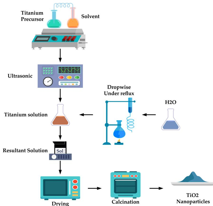
Figure 5. Scheme of the preparation of TiO<sub>2</sub> nanoparticles via sol-gel.
