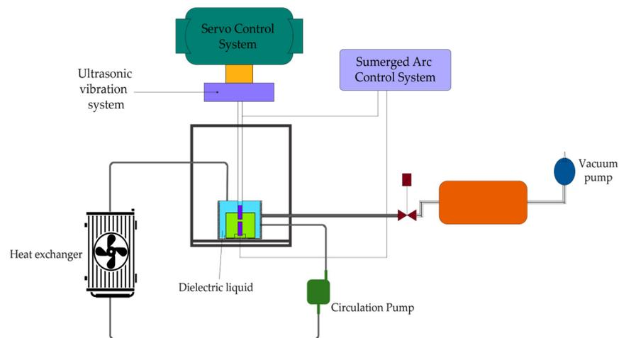
**Figure 3.** Schematic diagram of a submerged arc nanoparticle synthesis system.
