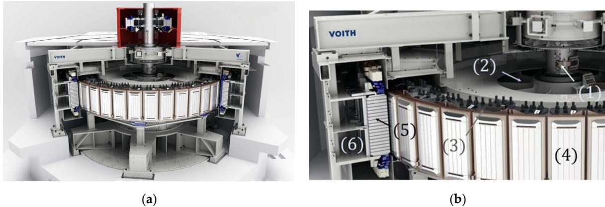
**Figure 1.** (a) Model of a hydropower generator. (b) Different parts of the generator: (1) shaft; (2) rotor spider; (3) rotor rim; (4) poles; (5) stator core; (6) stator frame. Reproduced with permission from Voith Hydro AB.
