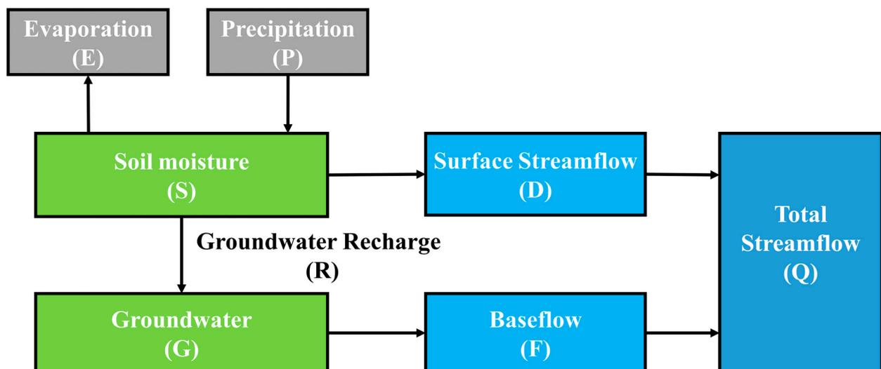
Figure 3. Conceptual diagram of the ABCD model.
