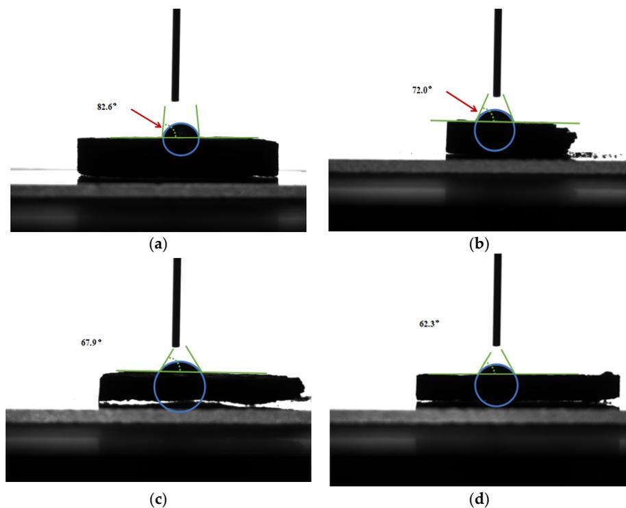
**Figure 2.** Schematic diagrams of contact angles of coal samples: (a) raw coal; (b) coal treated with 1 wt% [Bmin]Cl solution; (c) coal treated with 3 wt% [Bmin]Cl solution; (d) coal treated with 5 wt% [Bmin]Cl solution.
