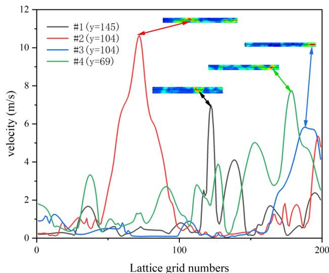
**Figure 6.** Velocity profile of the seepage channel of each coal sample.
