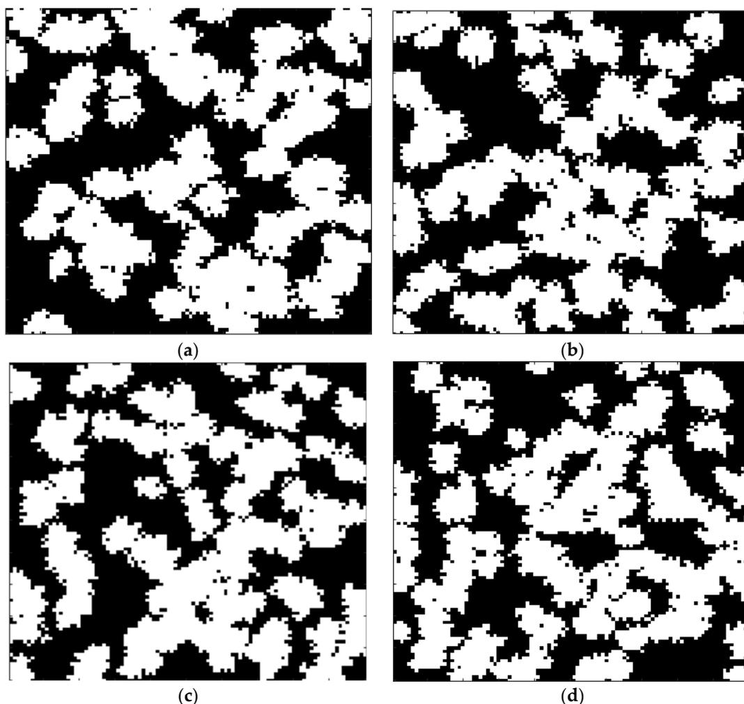
**Figure 3.** Schematic diagrams of the pore reconstruction of coal samples: (a) raw coal; (b) coal treated with 1 wt% [Bmin]Cl solution; (c) coal treated with 3 wt% [Bmin]Cl solution; (d) coal treated with 5 wt% [Bmin]Cl solution.
