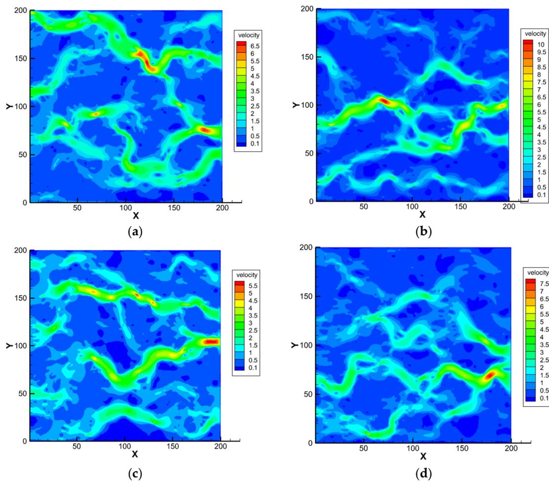
**Figure 4.** CO<sub>2</sub> velocity distribution of each coal sample presented in an LBM simulated cloud map: (a) raw coal; (b) coal treated with a 1 wt% [Bmin]Cl solution; (c) coal treated with a 3 wt% [Bmin]Cl solution; (d) coal treated with a 5 wt% [Bmin]Cl solution.
