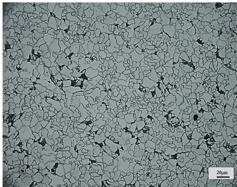
**Figure 1.** Microstructure diagram of L360 steel. Magnification: 500 $\times$ .
