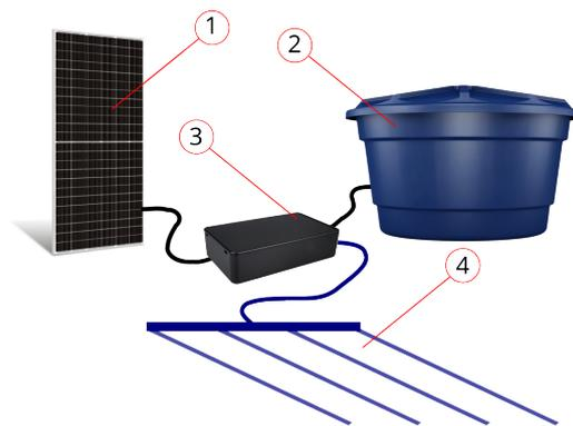
**Figure 3.** Simplified arrangement of irrigation system components, consisting of (1) photovoltaic panels, (2) water reservoirs, (3) the assembled prototype, and (4) drip tapes.
