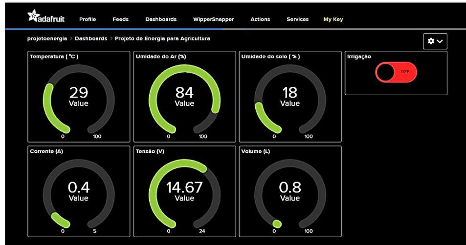
**Figure 6.** Visualisation of readings taken by sensors through the dashboard developed on the Adafruit IO platform.
