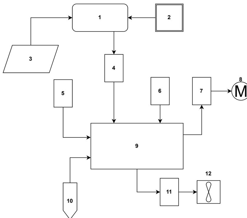
**Figure 1.** Automated, solar-powered irrigation prototype connections. (1) PWM ECP 1024 Intelbras charge controller; (2) battery; (3) 85 W poly R5A/D solar panel; (4) 25 V voltage sensor, ACS712 5A current sensor; (5) humidity and temperature sensor—DHT11; (6) ESP8266 development board; (7) 5 V relay module—two channels; (8) motor pump; (9) Arduino Uno R3; (10) resistive soil moisture sensor; (11) 5 V relay module—two channels; (12) flow sensor model YF-S201.
