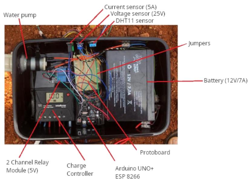
**Figure 2.** Practical assembly of the irrigation prototype.
