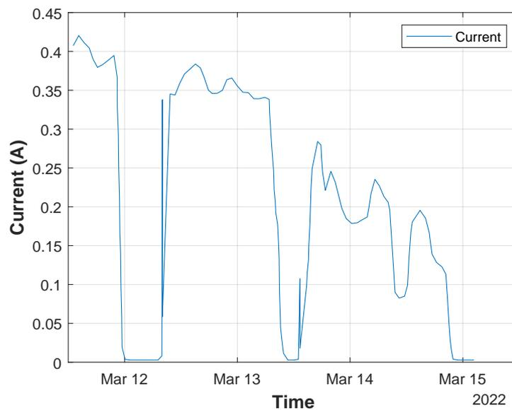
Figure 16. Readings taken by the ACS712 5th current sensor.
