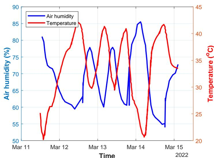
Figure 20. Air temperature and humidity readings—DHT 11.
