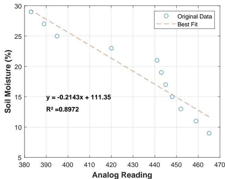
**Figure 5.** Calibration of the HL-69-resistive soil moisture sensor.
