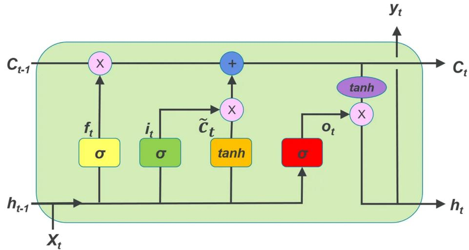
Figure A1. LSTM architecture.
