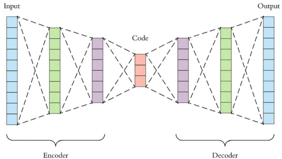
**Figure 1.** A general autoencoder architecture.
